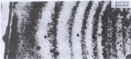
Figure 6. Acoustic image of a brass-epoxy-brass joint (thickness of each brass sheet is 6 mils, thickness of epoxy layer varies from 1.5 mils at one end to 4.5 mils at the other).
