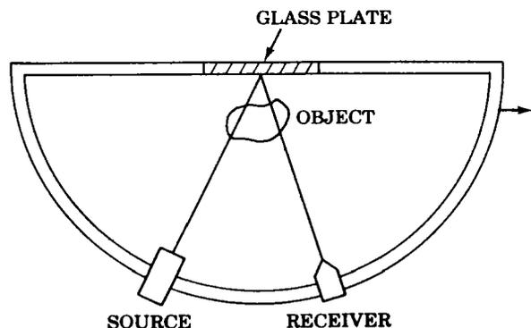
Figure 1. Experimental arrangement for reflection tomographic imaging.
