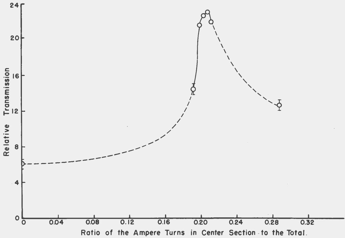
Fig. 13 - Relative transmission versus the ratio of ampere-turns in the three coils.
