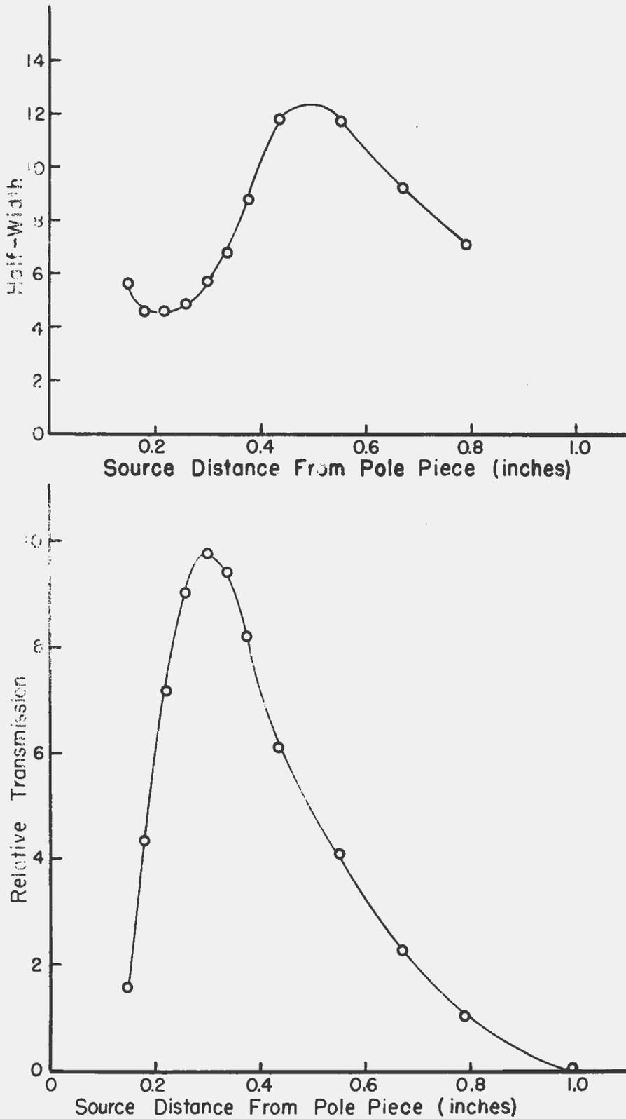
Fig. 14 - Transmission and half-width as a function of source position (with counter position fixed).
