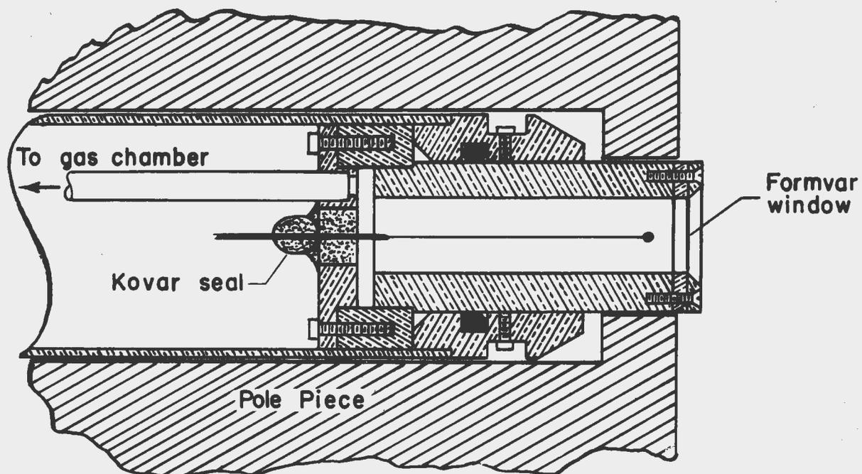
Fig. 17 - Arrangement of Geiger counter used in preliminary adjustments.
