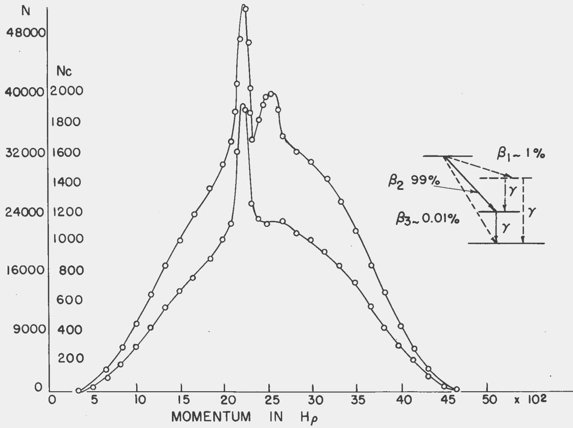
Fig. 20 - Total and coincidence spectra of  $Au^{198}$ .
