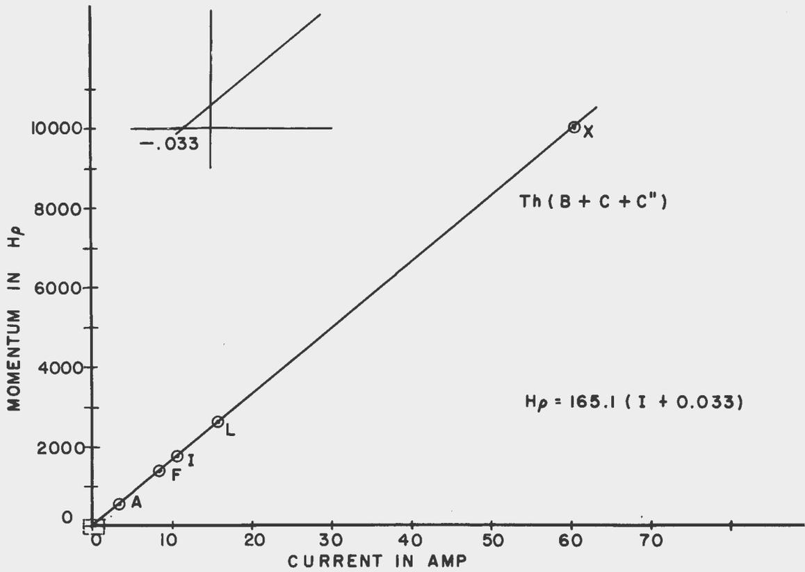
Fig. 19 - Calibration curve of spectrometer from conversion lines in Th(B+C+C'').
