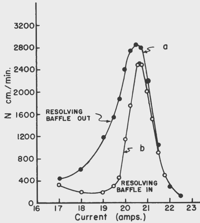
Fig. 16 - Effect of resolving baffle on line spectrum.
