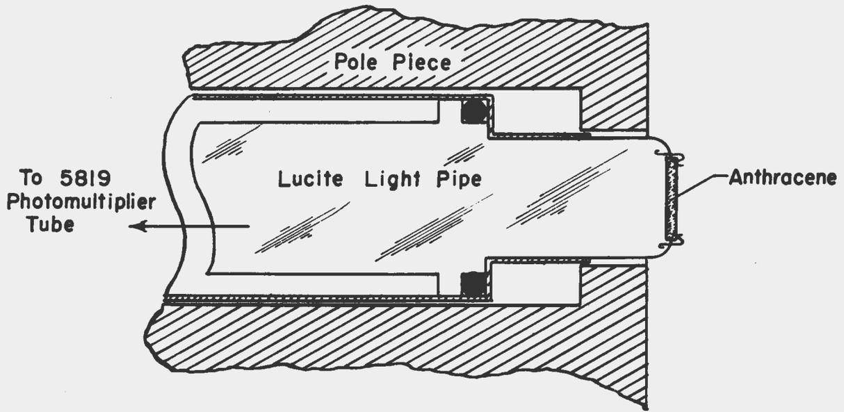
Fig. 8 - Anthracene crystal and Lucite pipe for beta-ray counter.
