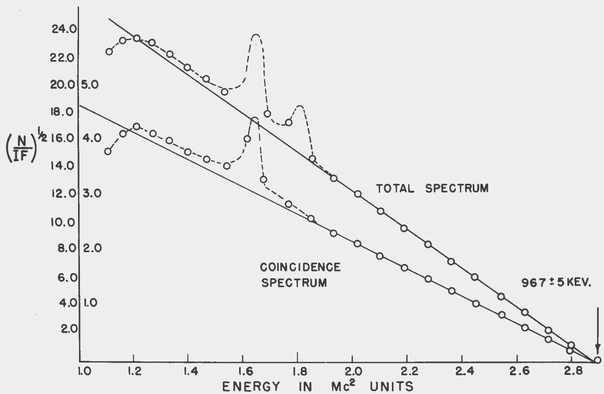
Fig. 21 - Kurie plots of total and coincidence spectra of Au<sup>198</sup>.
