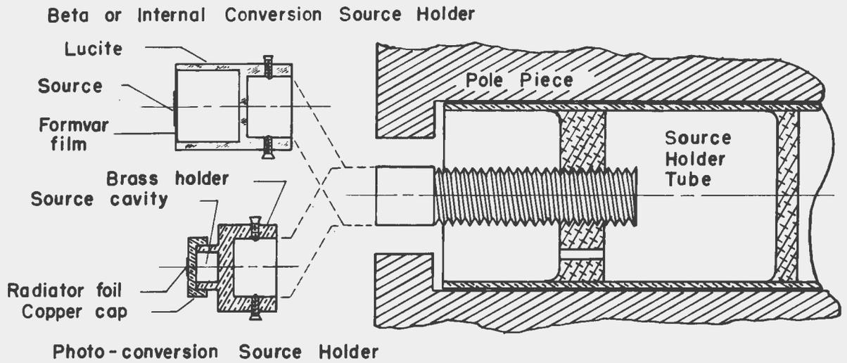
Fig. 7 - Source holders and positioning in spectrometer.
