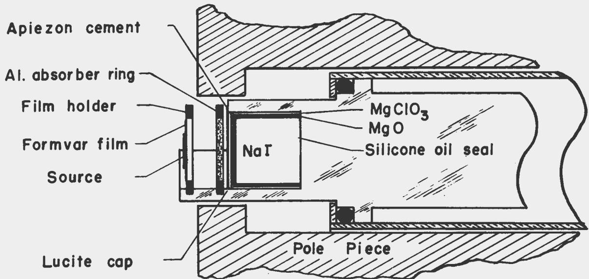
Fig. 9 - Arrangement of source and crystal of gamma-ray counter for coincidence measurements.
