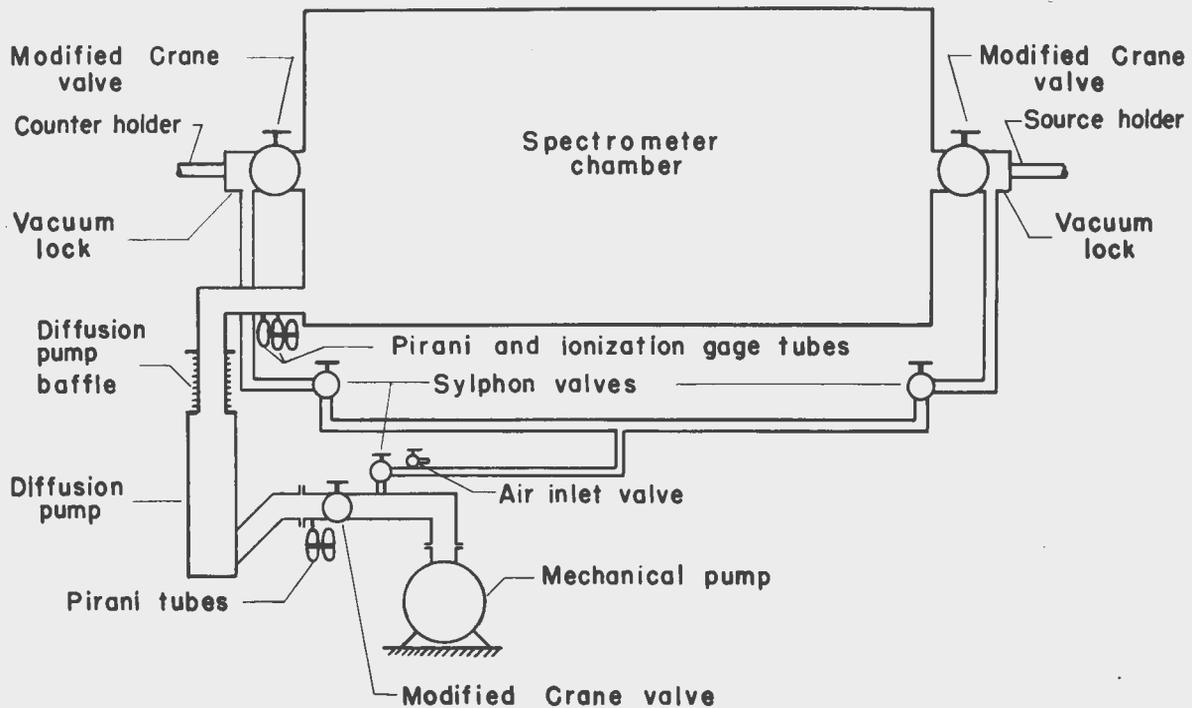
Fig. 6 - Schematic view of the vacuum system.
