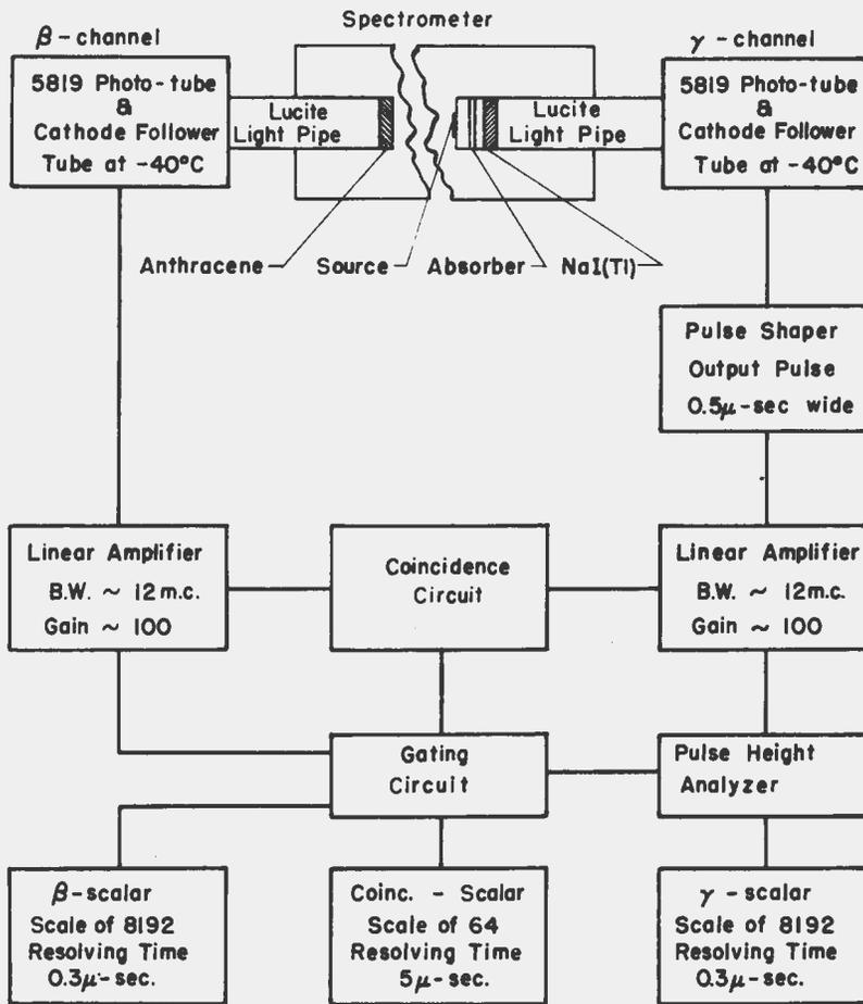
Fig. 10 - Block diagram of counting circuits.
