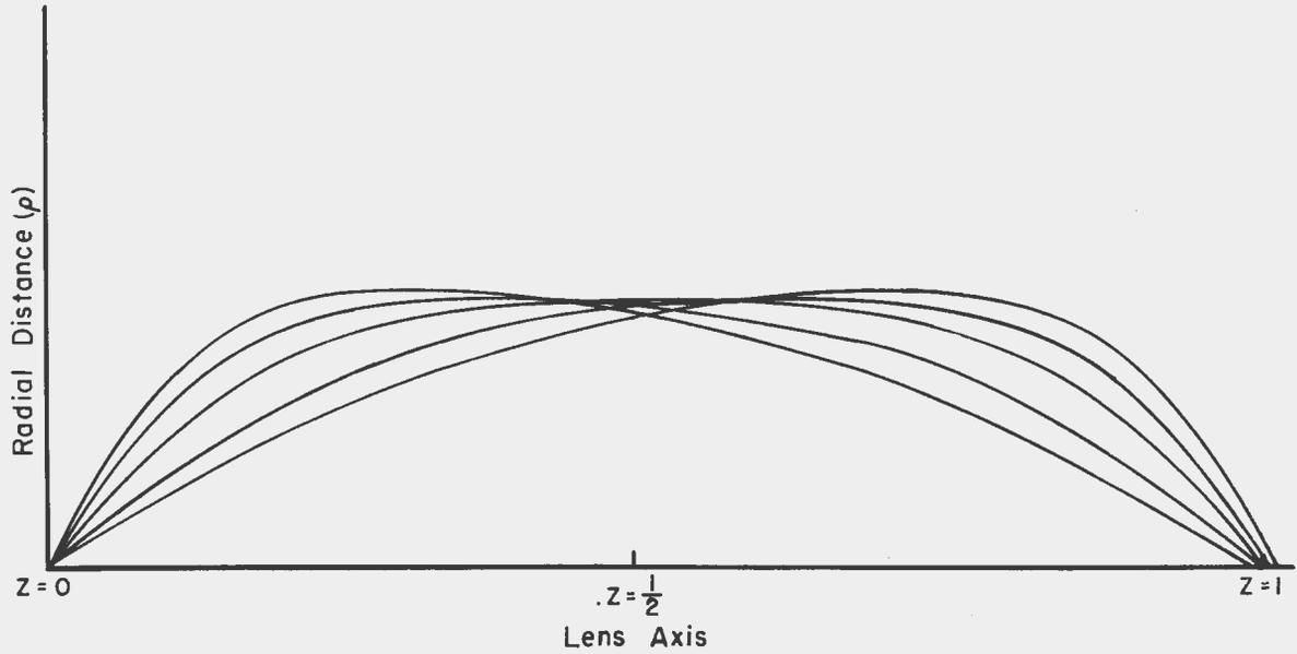
Fig. 3 - Trajectories of monoenergetic electrons in an intermediate image beta-ray spectrometer.
