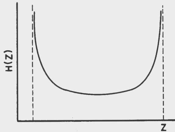
Fig. 1 - Magnetic field form for zero spherical aberration as calculated by W. Glaser.
