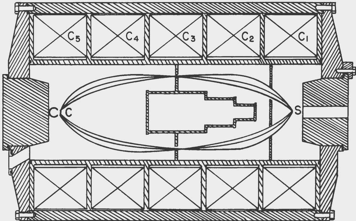
Fig. 2 - Schematic axial cross section of the intermediate image beta-ray spectrometer of Slatis and Siegbahn.
