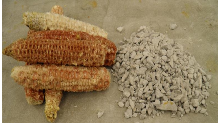
Figure 1. Use of limestone fines and corn cobs as raw materials to make soluble calcium
