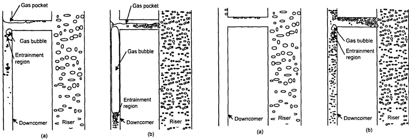
**Figure 2.** Gas pocket and bubble locations in the ELALR when the downcomer vent is closed (mode CV): (a) restrict flow regime ( $U_G = 0.5 \text{ cm/s}$ ) and (b) fully restricted flow regime ( $U_G = 20 \text{ cm/s}$ ).
