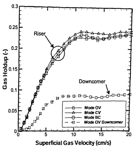
Figure 5. Effect of ELALR operation mode on gas holdup for  $A = 0.62\%$ .
