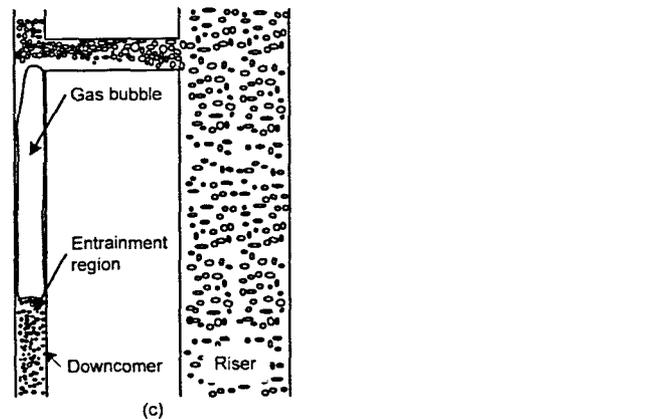
**Figure 3.** Gas bubble location in the ELALR when the downcomer vent is open (mode OV): (a) unrestricted flow regime ( $U_G = 0.5 \text{ cm/s}$ ), (b) restricted flow regime ( $U_G = 3.5 \text{ cm/s}$ ), and (c) fully restricted flow regime ( $U_G = 20 \text{ cm/s}$ ).
