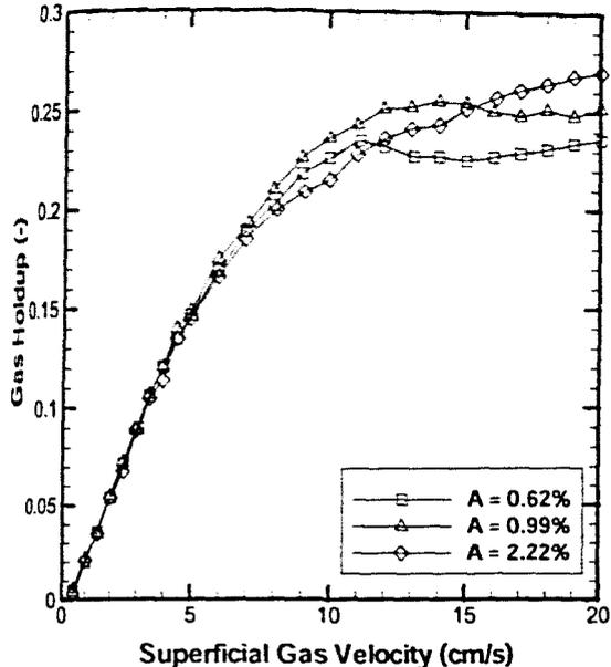
Figure 4. Gas holdup using different aeration plates when the ELALR is operated in mode BC.
