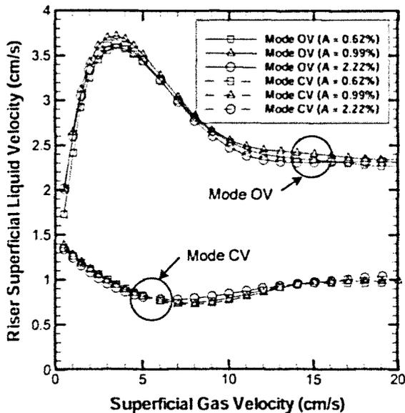
Figure 7. Aerator plate open area ratio and mode of operation effects on  $U_{Lr}$ .
