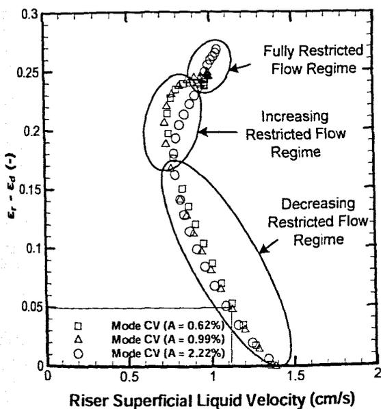
Figure 9. Relationship between driving force ( $\epsilon_r - \epsilon_d$ ) and  $U_{Lr}$  as a function of aerator plate open area ratio for mode CV ELALR operation.
