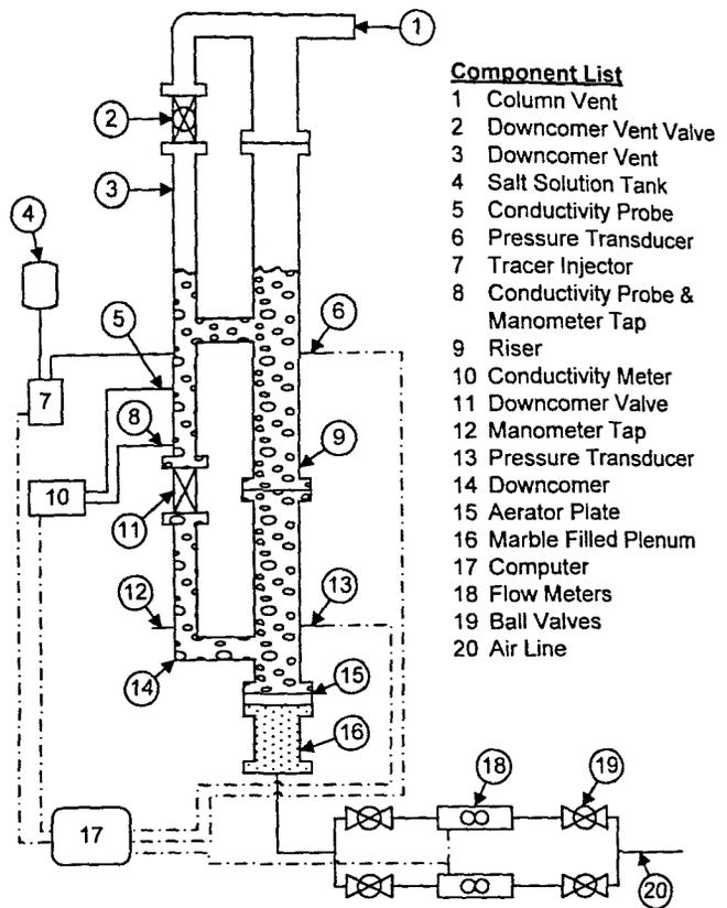
Figure 1. Experimental external loop airlift reactor schematic.
