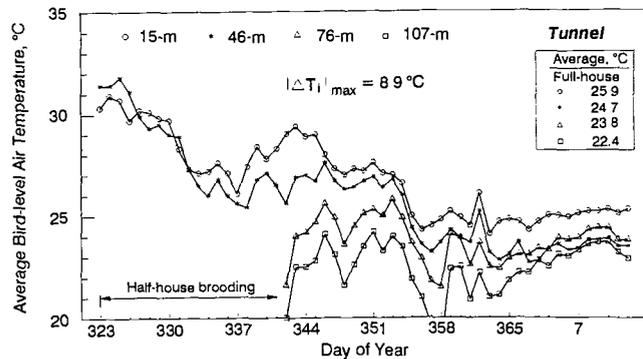
**Figure 4—Lengthwise temperature patterns of the experimental broiler houses during the winter flock (Legends of 15 m, 46 m, 76 m, and 107 m represent distances of the sensors from the east end of the house.  $T_i = 15\text{-m, } 46\text{-m, } 76\text{-m, and } 107\text{-m bird-level temperature. } ft = 3.28 \times m. \text{ } ^\circ F = 32 + ^\circ C \times 1.8).$**
