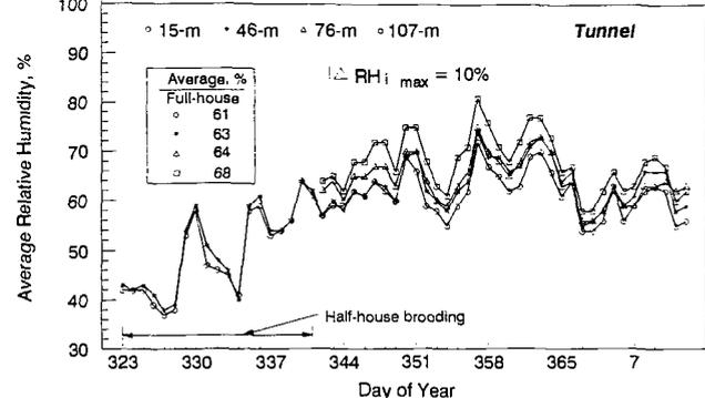
**Figure 5—Lengthwise RH patterns of the experimental broiler houses during the winter flock (Legends 15 m, 46 m, 76 m, and 107 m represent distances of the sensors from the east end of the houses.  $RH_i = 15\text{ m, } 46\text{ m, } 76\text{ m, and } 107\text{-m RH. } ft = 3.28 \times m. \text{ } ^\circ F = 32 + ^\circ C \times 1.8).$**
