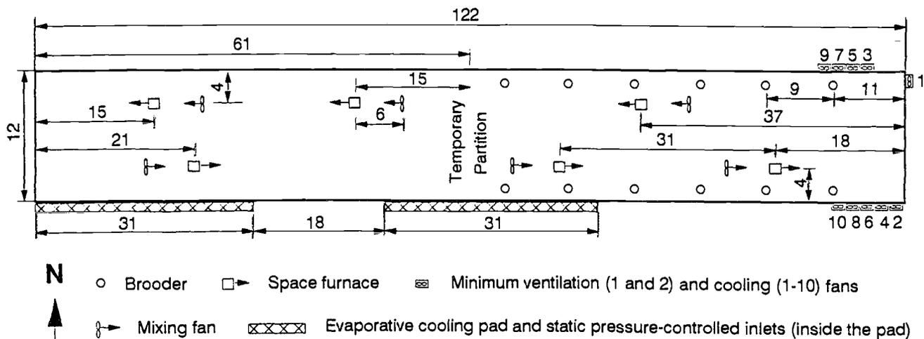
Figure 2—Schematic layout of the heating, cooling, and ventilating equipment of the experimental tunnel broiler houses. Side curtains used full length of building except over the two 31-m (100-ft) evaporative cooling pads (dimensions in meters – ft = m × 3.28).
