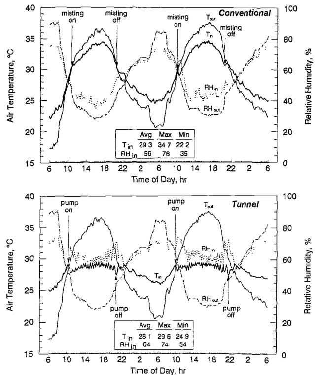
**Figure 7—Diurnal outside and inside air temperature (T) and RH patterns during two hot summer days. Operation of misting was continuous from on to off time, whereas pad cooling was cyclic as shown by the small temperature cycles. (Subscripts “out” and “in” represent outside and inside, respectively. ° F = 32 + ° C × 1.8).**
