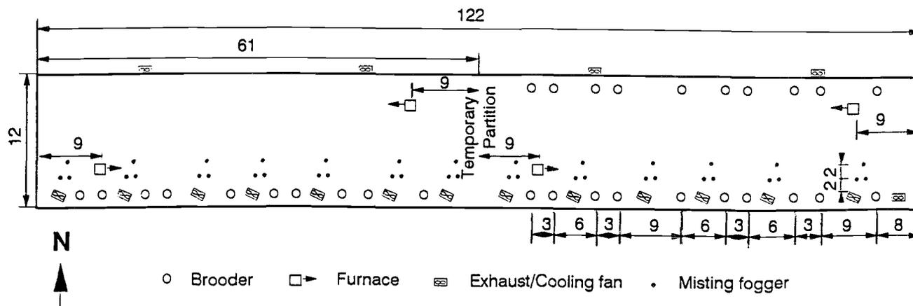
Figure 1—Schematic layout of the heating, cooling, and ventilating equipment of the experimental conventional broiler houses. Side curtains used full length of building (dimensions in meters – ft = m × 3.28).
