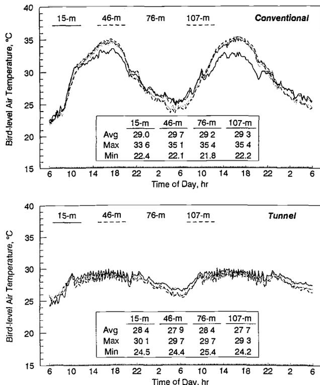
Figure 8—Lengthwise temperature patterns of the experimental broiler houses during two hot summer days (Locations of 15 m, 46 m, 76 m, and 107 m represent distances of the sensors from the east end of the house.  $ft = 3.28 \times m$ .  $^{\circ}F = 32 + ^{\circ}C \times 1.8$ ).
