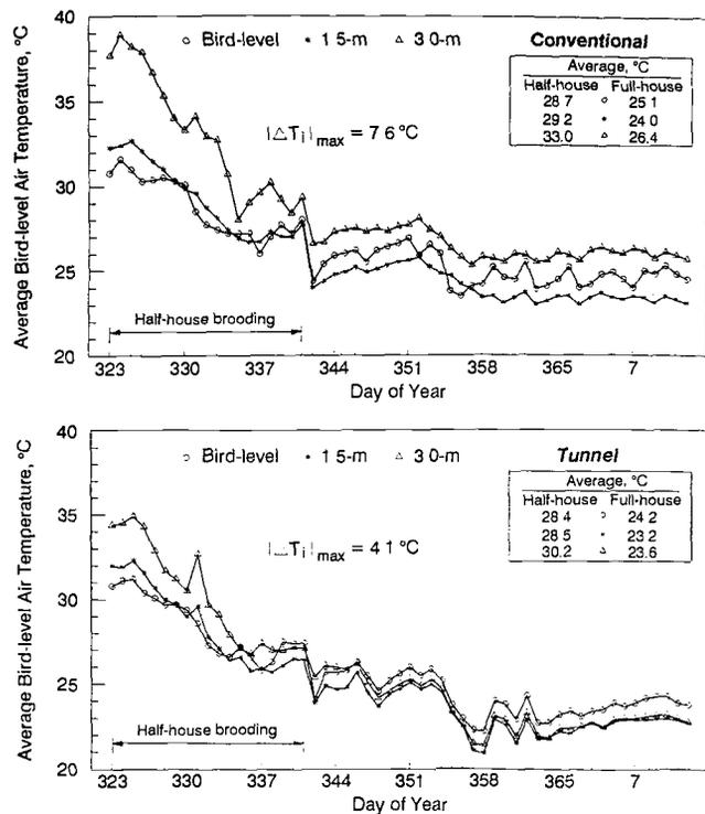
Figure 3—Vertical temperature patterns of the experimental broiler houses during the winter flock (Legends 1.5 m and 3.0 m represent distances of the sensors to the floor.  $T_i$  = bird-level, 1.5-m, and 3-m temperature.  $\text{ft} = 3.28 \times \text{m}$ .  $^{\circ}\text{F} = 32 + ^{\circ}\text{C} \times 1.8$ ).
