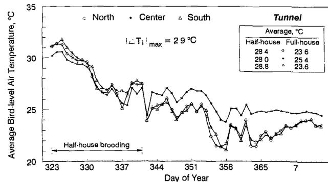
**Figure 6—Crosswise temperature patterns of the experimental broiler houses during the winter flock (Legends north, center, and south represent sensor locations that were 10.4 m, 6.1 m, and 1.8 m, respectively, from the south sidewall.  $T_i = \text{south, center, and north bird-level temperature. } ft = 3.28 \times m. \text{ } ^\circ F = 32 + ^\circ C \times 1.8).$**
