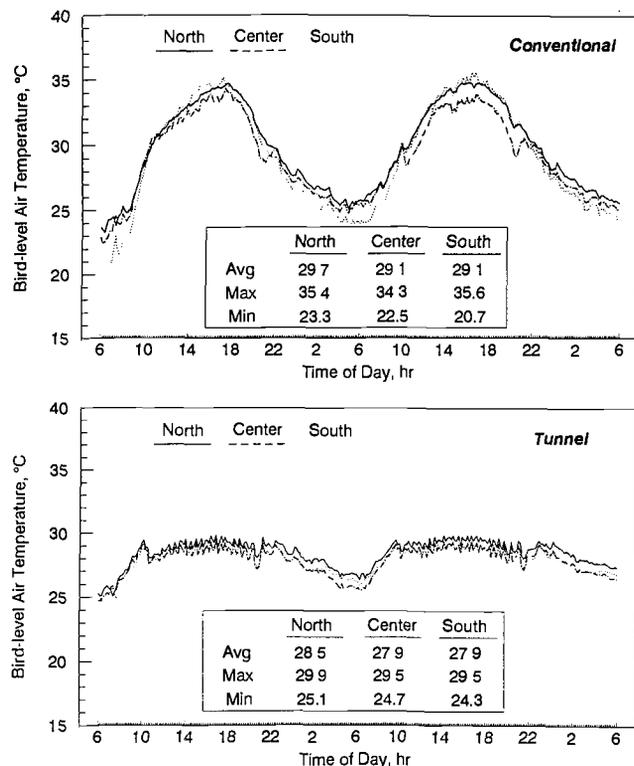
Figure 9—Crosswise temperature patterns of the experimental broiler houses during the two hot summer days (Legends north, center, and south represent sensor locations that were 10.4 m, 6.1 m, and 1.8 m, respectively, from the south sidewall.  $ft = 3.28 \times m$ .  $^{\circ}F = 32 + ^{\circ}C \times 1.8$ ).
