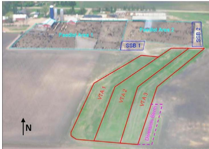
Figure 1. Layout of Central Iowa 1 and the VTS used to control and treat runoff generated by the facility.
