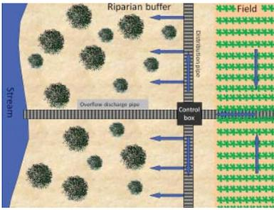
Overhead schematic of the buffer after creation of a saturated buffer.
