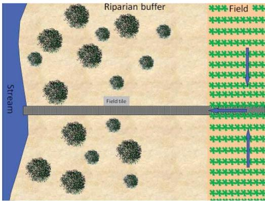
Overhead schematic of the buffer before creation of a saturated buffer.
