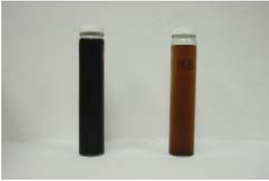
Suspended iron in the effluent.
