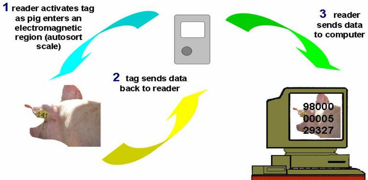
Figure 2. An illustration of the RFID mechanism.
