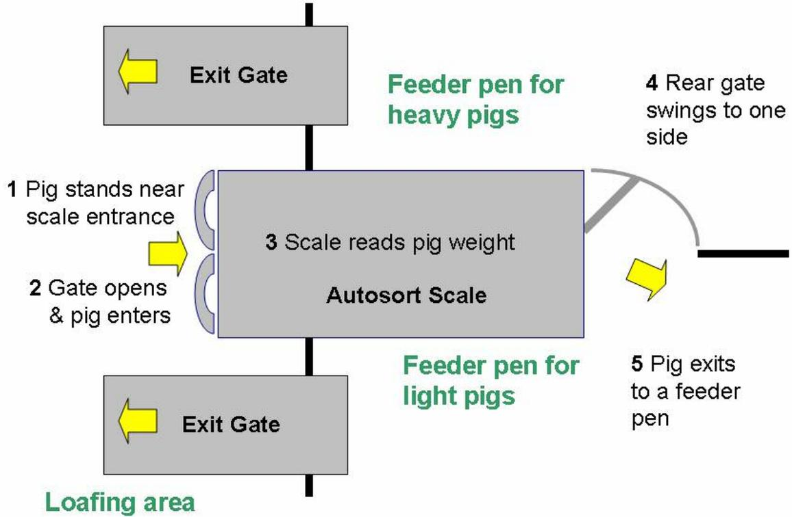
**Figure 3.** An illustration of the automatic sorting mechanism.
