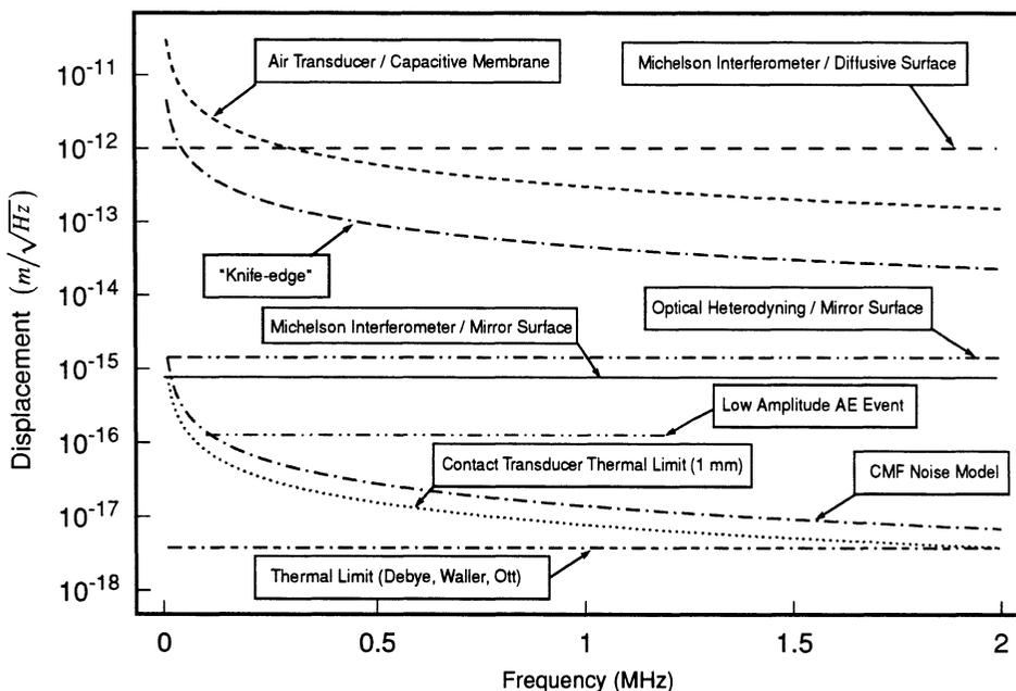
Figure 1. Sensitivities of various transducers, AE event level and thermal vibration limits
