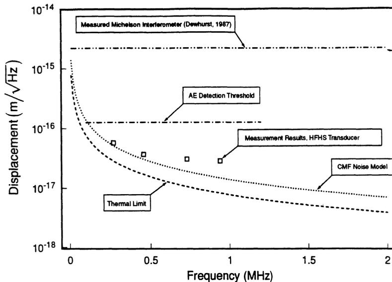
Figure 4. Measured minimum detectable displacement for the HFHS transducer.
