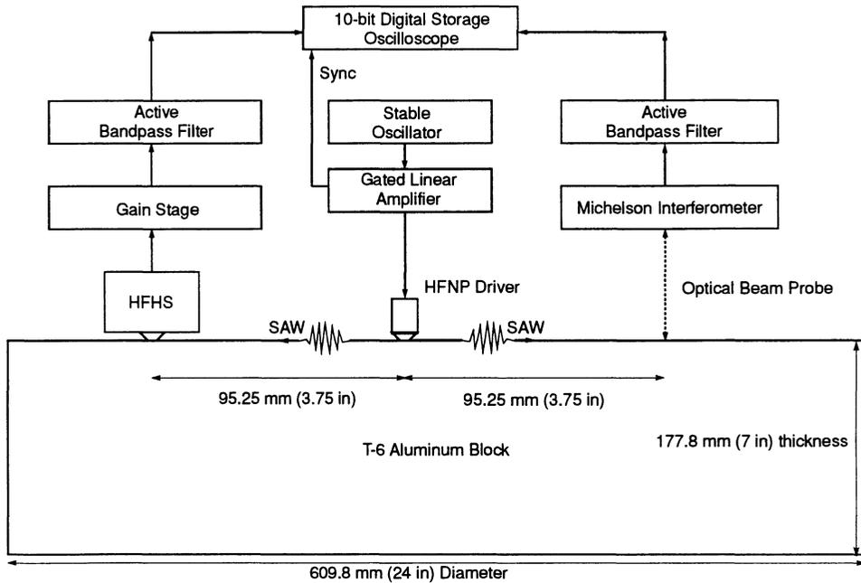
Figure 3. Displacement measurement configuration.
