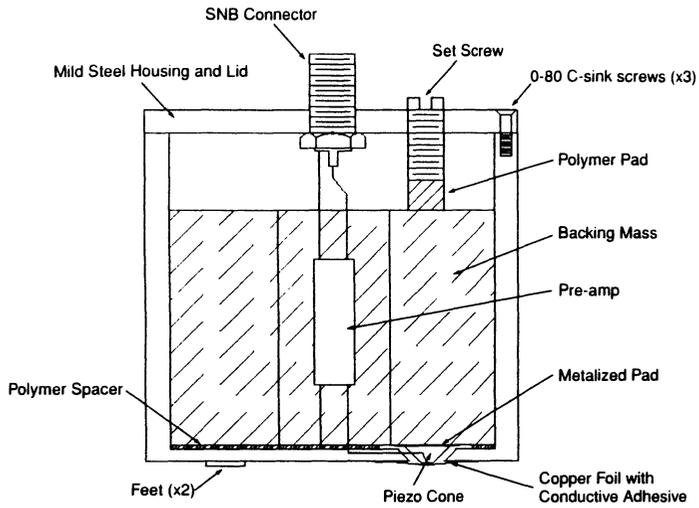
Figure 2a. Cross-section of HFHS direct-coupled transducer.
