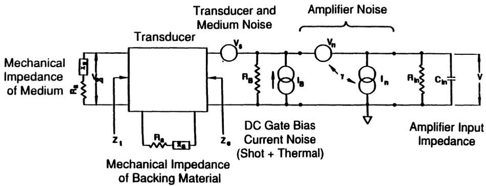
Figure 2b. Receiver front-end noise model.
