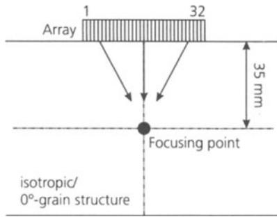
Figure 3. Modeling configuration: 32-element-array on top of a weld specimen. Point focusing is accomplished by time-delaying the single elements.
