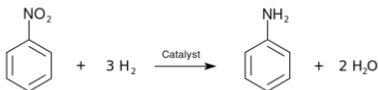
Scheme 2: Hydrogenation of nitrobenzene (Conditions: 1 mmol nitrobenzene, 0.3 mol % Fe, 10 bar H 2 , H 2 O: THF =1:1 (10 ml total volume), 120 °C, 3h)
