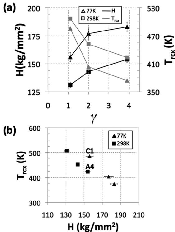
FIG. 1. Effect of shear strain ( $\gamma$ ) on hardness ( $H$ ) and recrystallization temperature ( $T_{\text{recx}}$ ). (b)  $T_{\text{recx}}$  as a function of  $H$ . Standard deviation for temperature was small ( $<3$  K). Points A4 and C1 correspond to copper deformed at (298 K,  $\gamma \sim 4$ ) and (77 K,  $\gamma \sim 1$ ), respectively.
