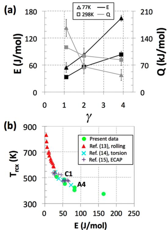
FIG. 2. (Color online) (a) Effect of shear strain ( $\gamma$ ) on stored energy ( $E$ ) and activation energy ( $Q$ ). (b) Recrystallization temperature ( $T_{\text{recx}}$ ) as a function of  $E$ . Points A4 and C1 correspond to copper deformed at (298 K,  $\gamma \sim 4$ ) and (77 K,  $\gamma \sim 1$ ), respectively.
