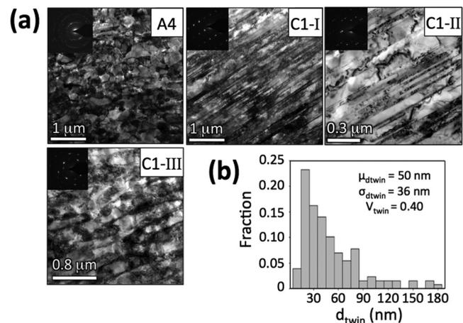
FIG. 3. (a) Representative micrographs of copper deformed at 298 K and  $\gamma \sim 4$  (inset A4), 77 K and  $\gamma \sim 1$  (insets C1-I to C1-III). (b) Histogram of twin spacing for copper deformed at 77 K and  $\gamma \sim 1$ .
