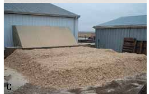
Figure 3. (A) Circular vertical biofilter; (B) rectangular vertical biofilter; and (C) flat-bed biofilter
