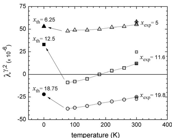
FIG. 1. Temperature dependence of the tetragonal magnetostriction of the three  $\text{Fe}_{100-x}\text{Si}_x$  samples studied (clear symbols); 300 K data from Ref. 7 is added, in both slow cooled (crossed symbols) and quenched (dotted symbols) states. The filled symbols represent 0 K theoretical results<sup>8</sup> at the compositions closest to the experimental ones.
