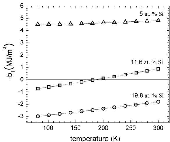
FIG. 3. Temperature dependence of the tetragonal magnetoelastic coupling,  $-b_1 = 2\lambda^2 c'$ , of Fe-Si at the three compositions studied.
