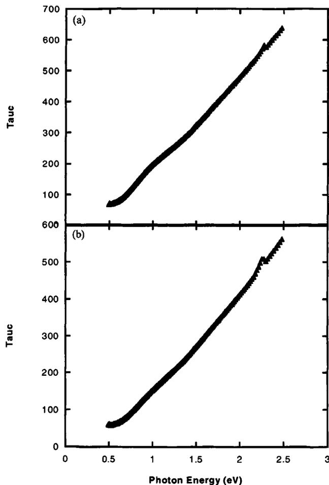
FIG. 3. Tauc plots of (a) the room-temperature-deposited Si-doped AlMgB<sub>14</sub> film and (b) the 573 K-deposited Si-doped AlMgB<sub>14</sub> film. The small peak in each plot is an absorption feature of the Corning 7059 glass.
