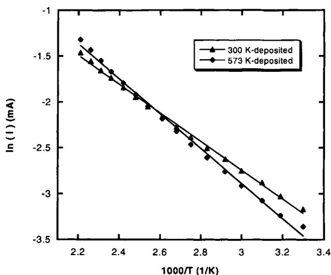
FIG. 1.  $\ln I$  vs  $1/T$  for the room-temperature- and 573 K-deposited Si-doped AlMgB<sub>14</sub> films.
