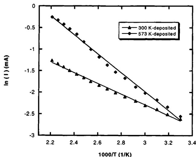
FIG. 2.  $\ln I$  vs  $1/T$  for the room-temperature- and 573 K-deposited baseline Si-free AlMgB<sub>14</sub> films.
