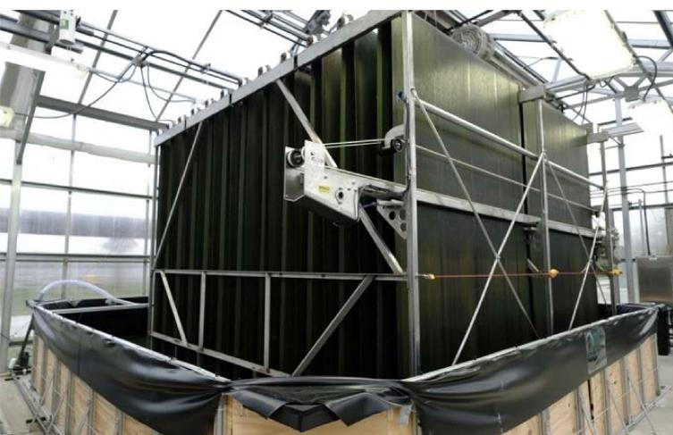
The figure above is one full-scale RAB reactor with the automatic harvester.
