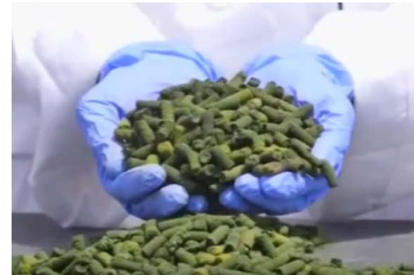
The figure seen above is a pelletized form of the algal after the harvest and drying processes.
