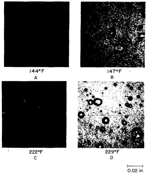
Figure 12. Photomicrographs of trapped air during resin cure ( $\theta = 0$ )
