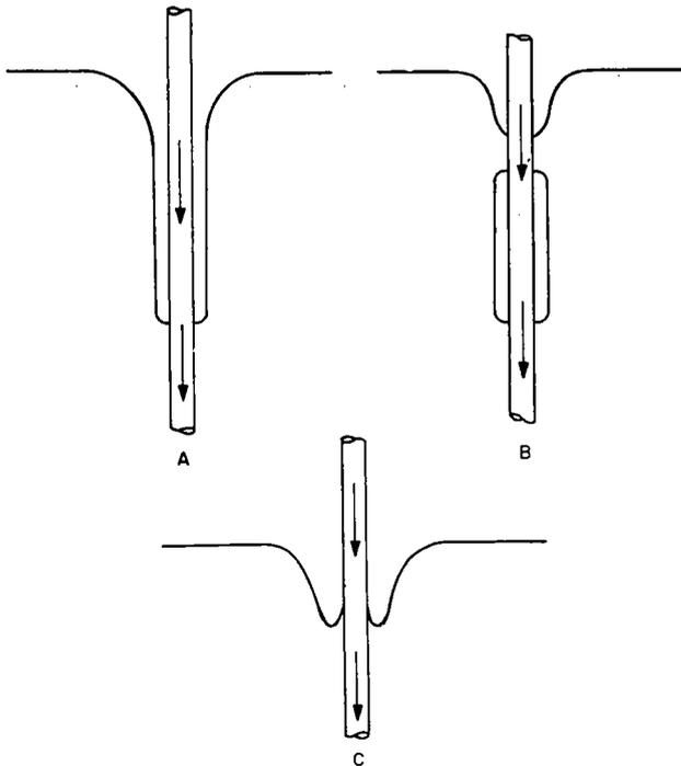
Figure 4. Schematic of air entrapment around a rod entering a liquid bath.
