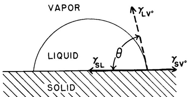
Figure 1. Equilibrium contact angle,  $\theta$ .  $\gamma_{LV}$  = liquid surface energy,  $\gamma_{SV}$  = solid surface energy and  $\gamma_{SL}$  = solid/liquid surface energy.
