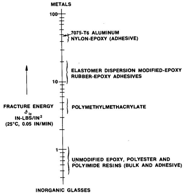
Figure 19. Ranking of  $\mathcal{G}_{Ic}$  ( $1 \text{ in-lb/in}^2 = 175.3 \text{ J/m}^2$ ).
