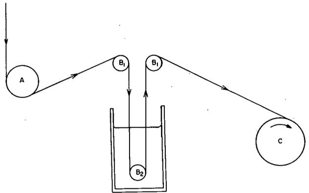
Figure 5. Experimental arrangement for observing air entrapment in filament winding. The strand is pulled from a spool (not shown) by the wind-up drum (C) and tension is maintained by a friction brake (A).
