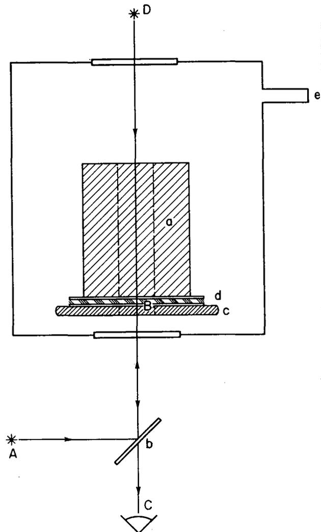
Figure 10. Experimental arrangement for viewing entrapped air at the adhesive/glass interface.
