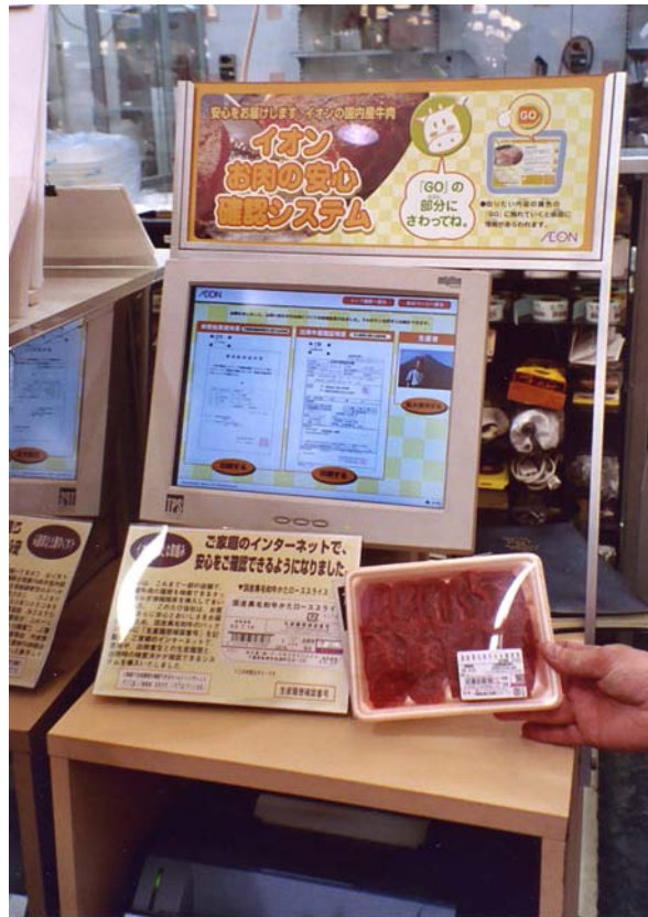
PHOTO 1. This computer in the meat department of a Jusco Supermarket (Aeon Company, Ltd.) is part of a Security Check System that allows customers to obtain information about the domestic Wagyu beef they are purchasing. Customers enter a 10-digit code from the meat package to obtain a production record (which provides full traceability to the producer), a government certificate of BSE testing, and a photograph of the producer(s). The customer could also obtain this information using a home computer.
