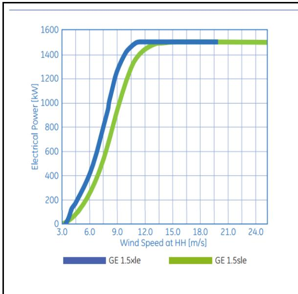
Figure 1: Power curve of a GE 1.5sle (green) and Ge 1.5xle (blue) wind turbine. (Adapted from (Moyer 2009)).
