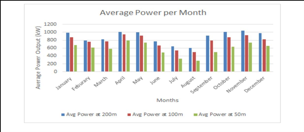
Figure 7: Determining the average monthly output of power for 200 m (blue), 100 m (red), 50 m (green) of the atmosphere.
