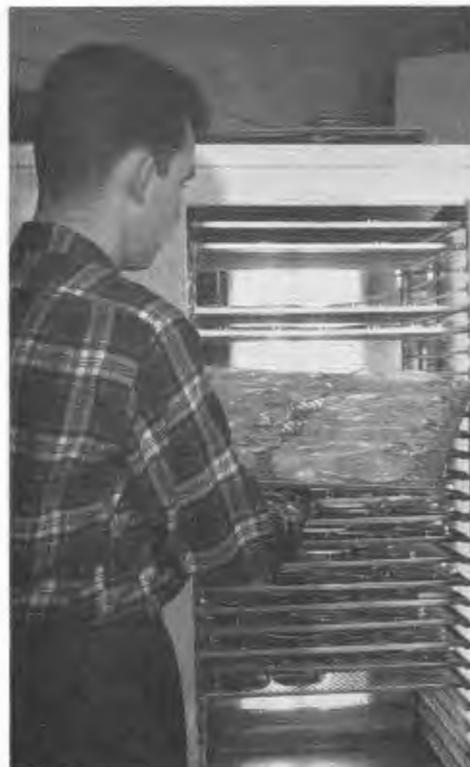
This photo shows a Stultz germinator used for germinating seed in covered petri dishes at the Seed Laboratory.
