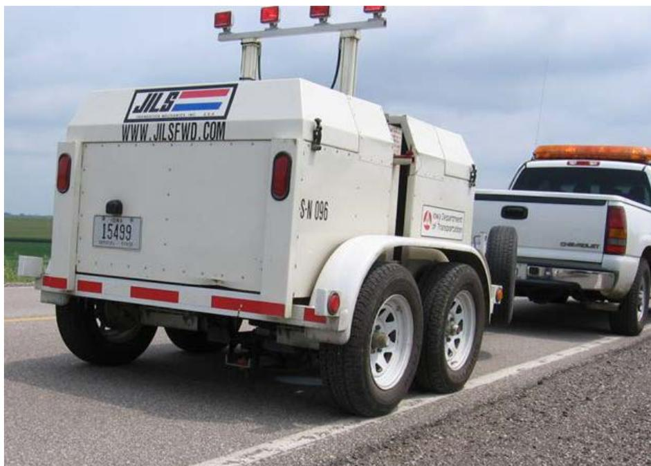
**Figure 1. Falling Weight Deflectometer (FWD)**
