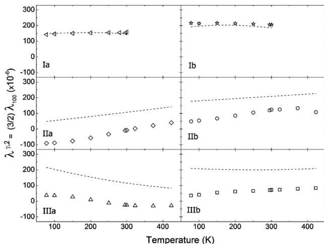
FIG. 1. Tetragonal magnetostriction  $(3/2)\lambda_{100}$  of  $\text{Fe}_{1-x-y}\text{Ga}_x\text{Ge}_y$  (SC) vs temperature (data points) and the corresponding weighted average (dotted line) from binary Fe–Ga (Ref. 3) and Fe–Ge (Ref. 1) data. The same scale is used for all graphs.
