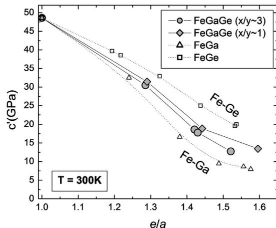
FIG. 3. Tetragonal shear modulus,  $c'$ , of  $\text{Fe}_{1-x-y}\text{Ga}_x\text{Ge}_y$  compared with  $c'$  of the binary Fe–Ga (Ref. 6) and Fe–Ge (Ref. 1) alloys vs electron-to-atom ratio,  $e/a$ , at 300 K (all data are from SC single crystals).
