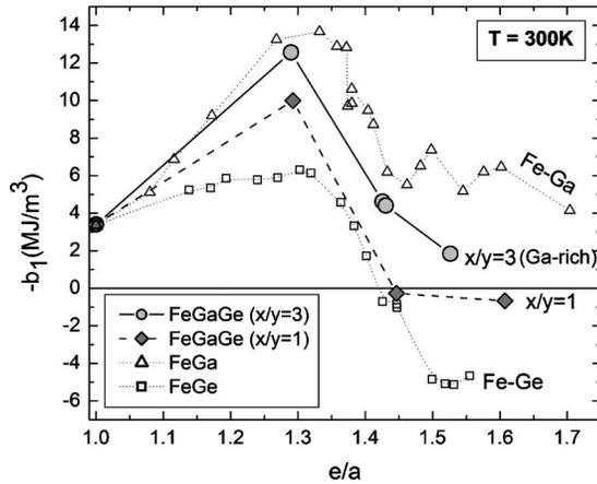
FIG. 4. Magnetoelastic coupling  $-b_1 = 3\lambda_{100}c'$  of  $\text{Fe}_{1-x-y}\text{Ga}_x\text{Ge}_y$  contrasted with those of the binary alloys Fe–Ga (Ref. 1) and Fe–Ge (Ref. 1) as a function of electron-to-atom ratio,  $e/a$ , at 300 K (all data are from SC single crystals).
