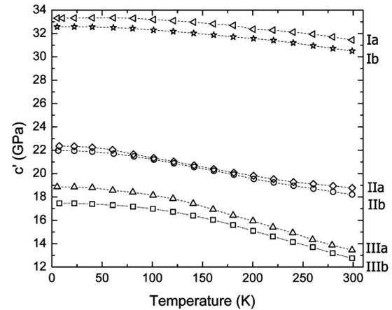
FIG. 2. Tetragonal shear modulus,  $c'$ , of the  $\text{Fe}_{1-x-y}\text{Ga}_x\text{Ge}_y$  single crystals (SC state) vs temperature.
