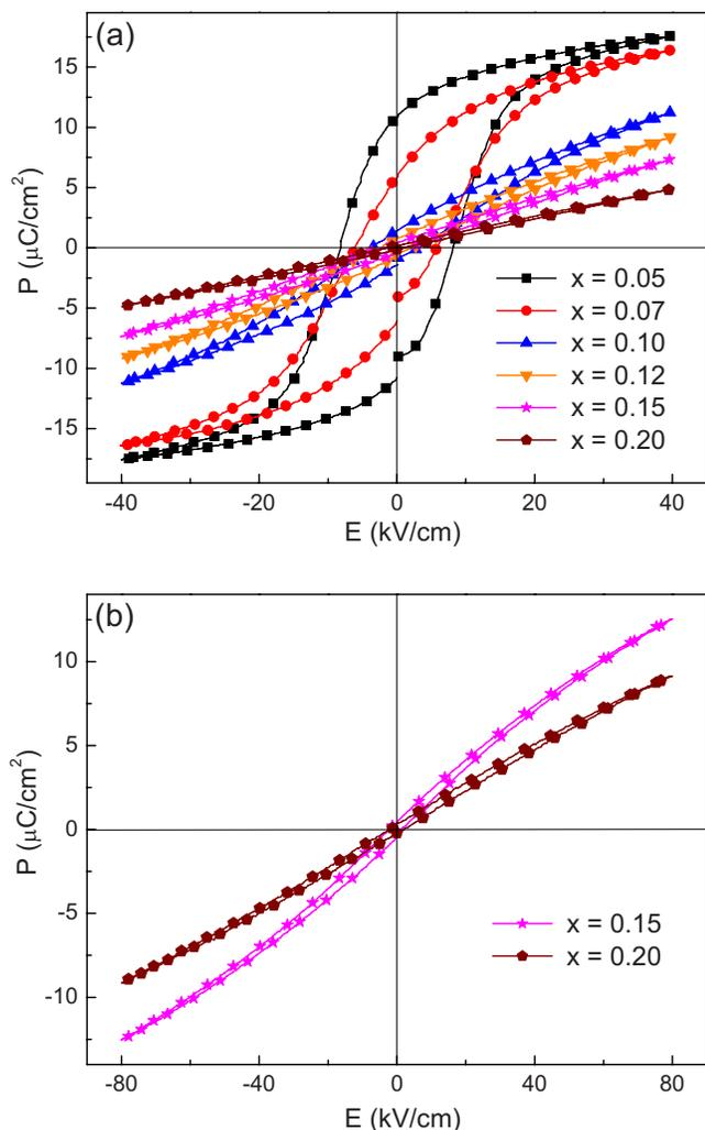
FIG. 5. (Color online) (a) Polarization  $P$  vs electric field  $E$  plots of  $(1-x)\text{BaTiO}_3-x\text{Bi}(\text{Li}_{1/3}\text{Ti}_{2/3})\text{O}_3$  ceramics measured at 4 Hz with 40 kV/cm peak field at room temperature. (b)  $P$  vs  $E$  plots for the composition  $x=0.15$  and 0.20 measured at 4 Hz with 80 kV/cm peak field at room temperature.
