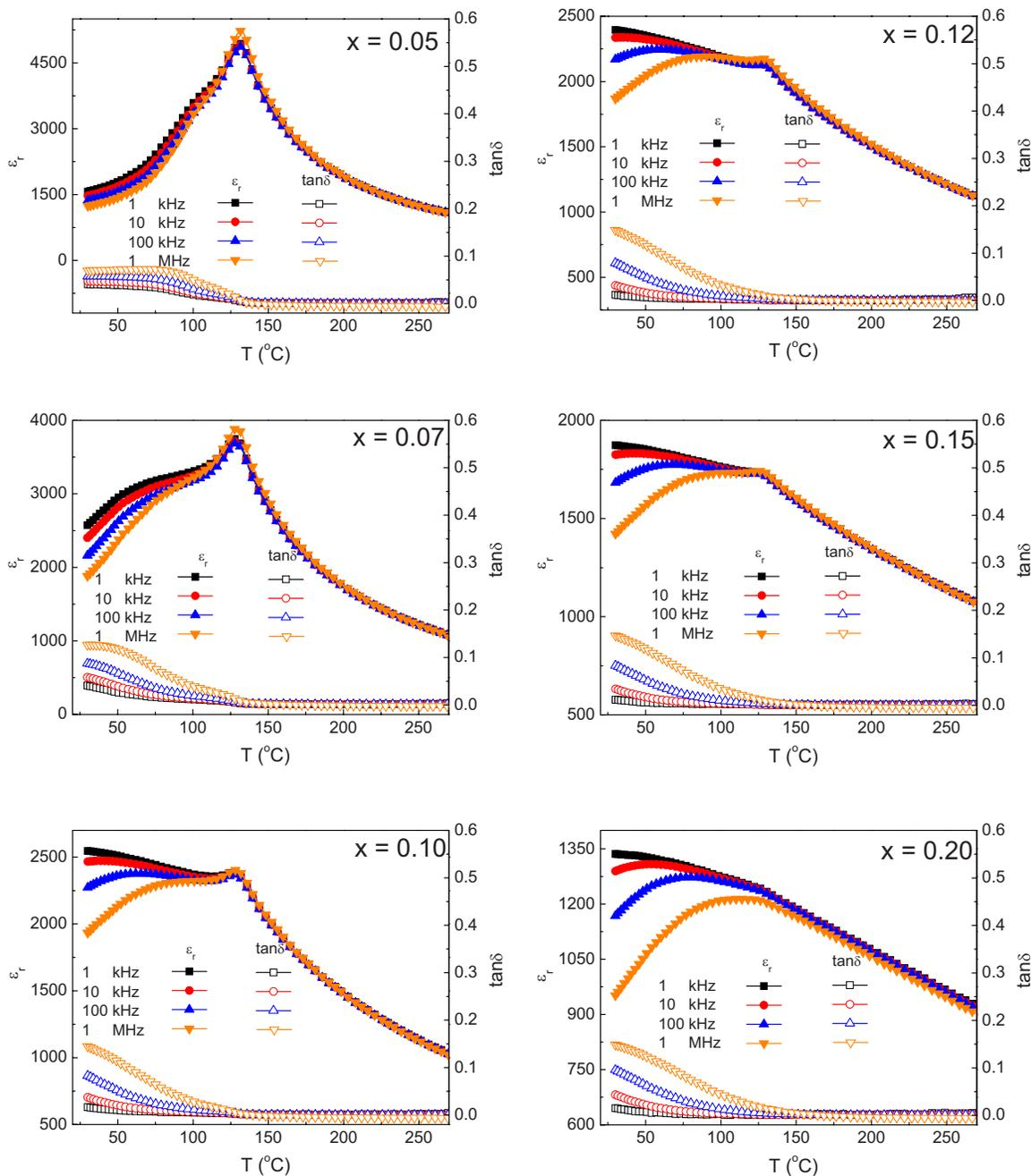
FIG. 2. (Color online) Temperature dependence of dielectric constant  $\epsilon_r$  and loss  $\tan\delta$  of  $(1-x)\text{BaTiO}_3-x\text{Bi}(\text{Li}_{1/3}\text{Ti}_{2/3})\text{O}_3$  ceramics measured at 1 kHz, 10 kHz, 100 kHz, and 1 MHz.
