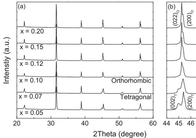
FIG. 1. XRD patterns of  $(1-x)\text{BaTiO}_3-x\text{Bi}(\text{Li}_{1/3}\text{Ti}_{2/3})\text{O}_3$  sintered samples in the range of  $2\theta$  (a) from  $20^\circ$  to  $60^\circ$  and (b) from  $44.0^\circ$  to  $46.5^\circ$ .
