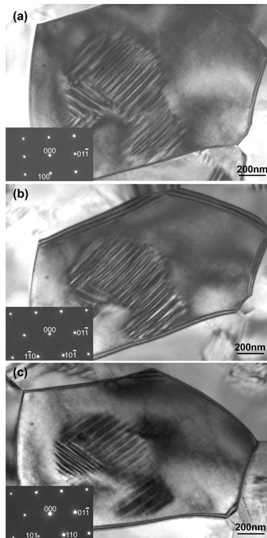
FIG. 4. TEM bright field images of a representative grain for  $x=0.10$  tilted to its (a)  $[011]$ , (b)  $[111]$ , and (c)  $[\bar{1}11]$  zone axes. The insets are the corresponding electron diffraction patterns.
