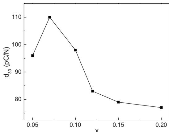
FIG. 6. The room temperature piezoelectric coefficient  $d_{33}$  as a function of composition  $x$  of  $(1-x)\text{BaTiO}_3-x\text{Bi}(\text{Li}_{1/3}\text{Ti}_{2/3})\text{O}_3$  ceramics.
