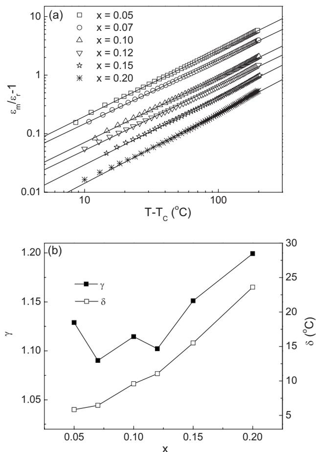
FIG. 3. (a) Plot of  $(\epsilon_m/\epsilon_r - 1)$  vs  $(T - T_c)$  in log scale using the  $\epsilon_r$  vs  $T$  data obtained at 1 MHz in the temperature range of 140–330 °C in  $(1-x)\text{BaTiO}_3 - x\text{Bi}(\text{Li}_{1/3}\text{Ti}_{2/3})\text{O}_3$  ceramics. The symbols represent the experimental data, while the solid lines are the linear fit. (b) The relaxation parameter  $\gamma$  and the diffuseness parameter  $\delta$  determined by the data fitting.
