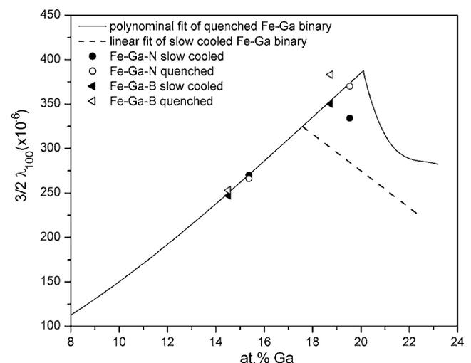
FIG. 2.  $(3/2) \lambda_{100}$  strain measurements as a function of Ga content for Galfenol with B and N additions together with the fitted binary data for comparison.
