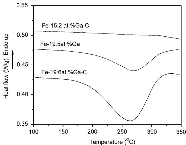
FIG. 3. Results of DSC scans of binary Fe–Ga and Fe–Ga–C quenched alloys with compositions as indicated. The released heats are 0.39 and 1.02 kJ/mol atom for Fe–Ga binary and Fe–Ga–C ternary alloys, respectively.
