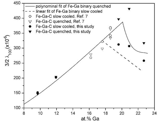
FIG. 1.  $(3/2) \lambda_{100}$  strain measurements as a function of Ga content for Galfenol with C additions together with the fitted binary data for comparison.
