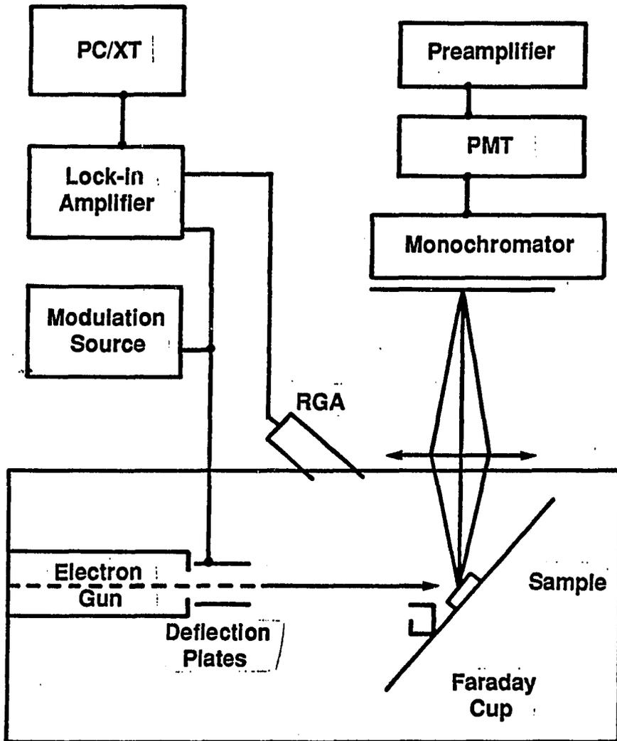
preamplifier/discriminator and a pulse counter, was used to measure the photon intensity. In this case, the background was mostly from the light emitted by the W filament of the electron gun, and it is also removed by modulating the electron beam.
