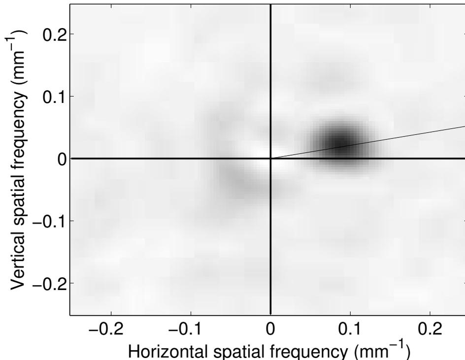
FIG. 4: Spatial Fourier transform of measured correlations, integrated from 200-300 kHz. The estimated direction of the leak is 12 deg from the horizontal.
