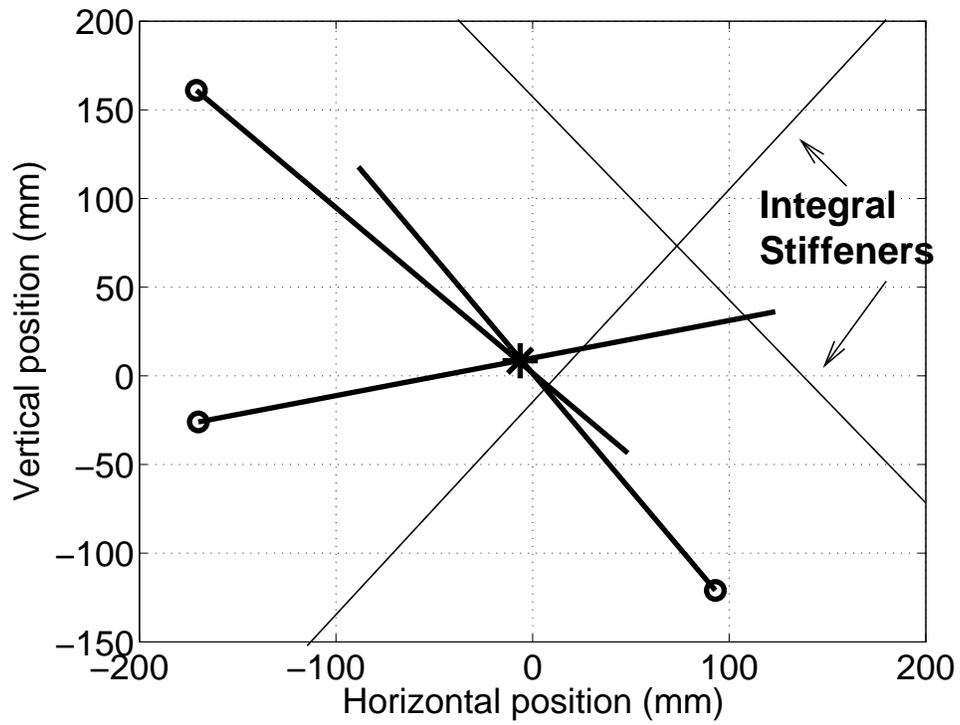
FIG. 5: Leak location and least-squares triangulation from three array locations ('o') to find the estimated leak location ('\*') at coordinates  $(-6.3, 8.5)$  mm. The actual location of the leak was the origin. Data from the sensors at coordinates  $(-175, -25)$  and  $(90, -120)$  are shown in Figs. 4 and 6 respectively.
