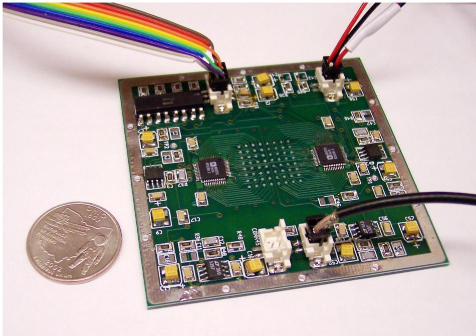
FIG. 1: Array sensor, showing electronics. A PZT disc element is placed under the grid at the center.
