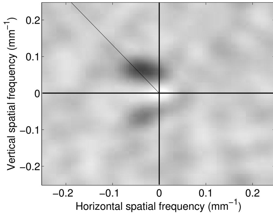
FIG. 6: Spatial Fourier transform of measured correlations, integrated from 200-300 kHz of the sensor shown in the lower right of Fig. 5.
