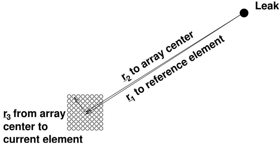
FIG. 2: Diagram showing  $\underline{r}_1$ ,  $\underline{r}_2$ , and  $\underline{r}_3$  relative to leak and sensor.
