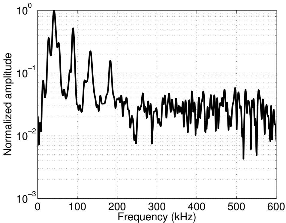
FIG. 3: Frequency spectrum of a leak noise cross-correlation. The peaks below 200 kHz are resonances within the PZT element.
