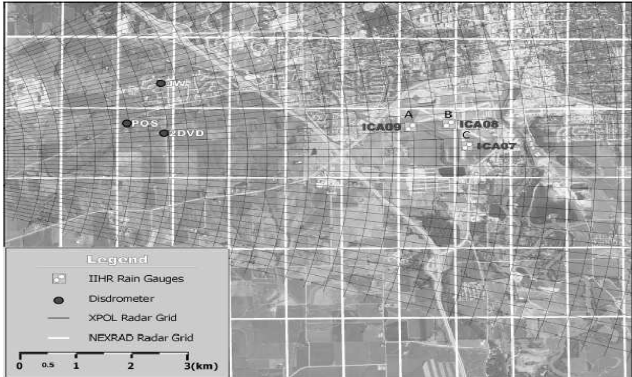
Fig. 1. Aerial photography of the experimental domain overlaid by the XPOL and nearest NEXRAD (KDVN) sampling grids, and of the dual-gauge and disdrometer locations. Photo courtesy of Anagnostou (2003).
