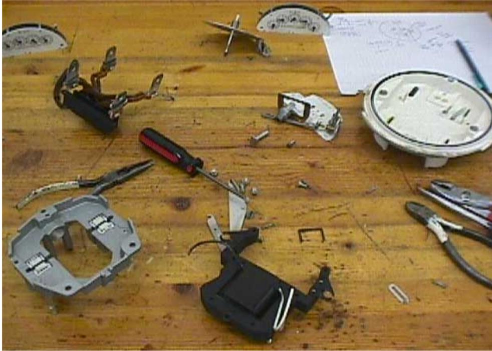
Figure 6. Disassembled watt-hour meter, showing major components
