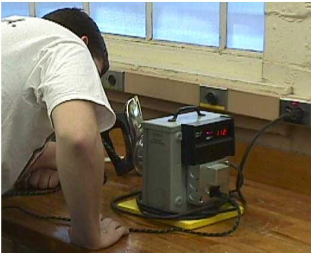
Figure 3. Power use measurement of a clothes iron using a watt-hour meter
