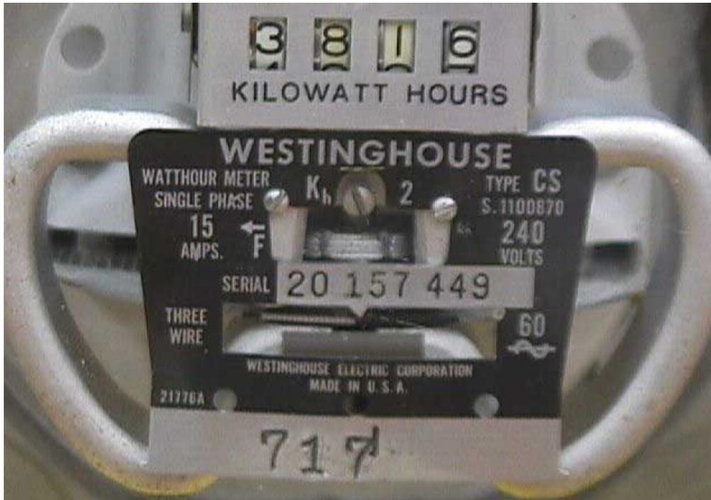
Figure 2. The faceplate of a Westinghouse watt-hour meter
