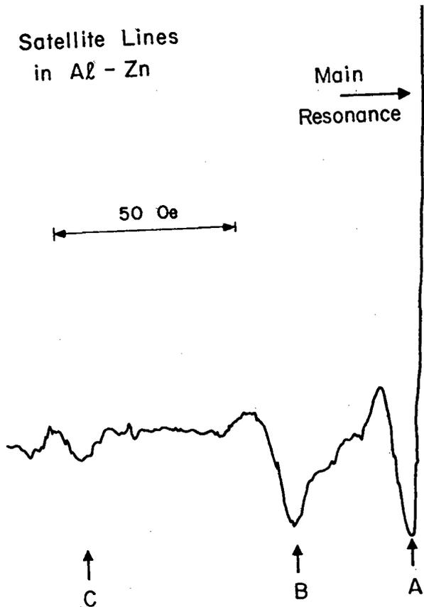
Figure 9. Acoustic Nuclear Resonance Signal from an Aluminum-Zinc Alloy
