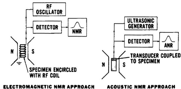
Figure 2 Experimental Methods for Nuclear Magnetic Resonance.
