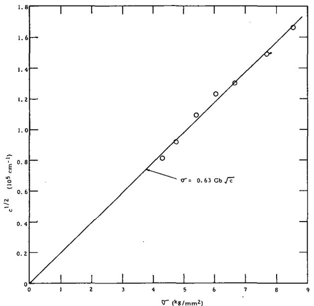
Figure 7. Square Root of the Mean Dislocation Density  $c$  in Polycrystalline Aluminum as Determined from NMR Signal Intensity Measurements versus Compressive Stress
