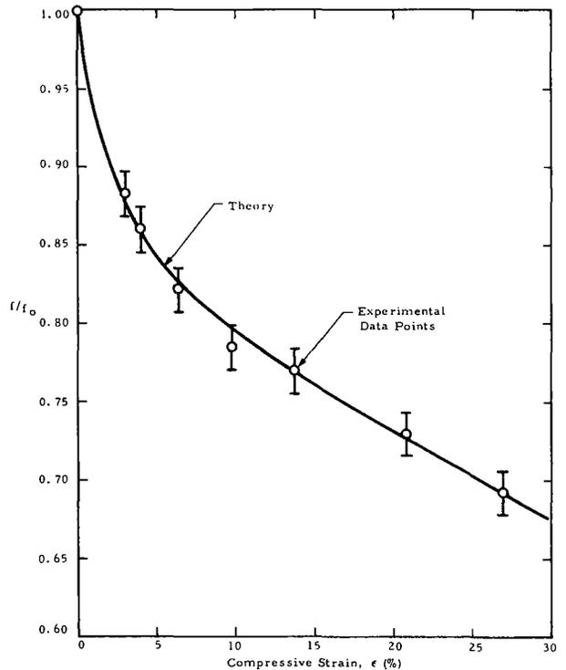
Figure 6. <sup>27</sup>Al Normalized Peak-to-Peak NMR Signal Intensity in Bulk Polycrystalline Aluminum versus Compressive Strain
