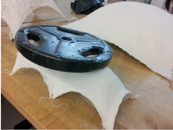
Figure 5: Testing of lightweight thin shell structures. This structure carries a load more than 100 times its dead load weight.
