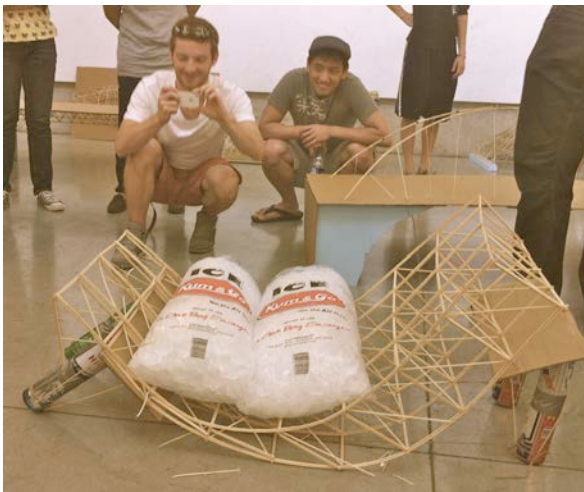
Figure 6: The box truss failure developed gradually under loading and failed progressively to the point of eventual collapse.
