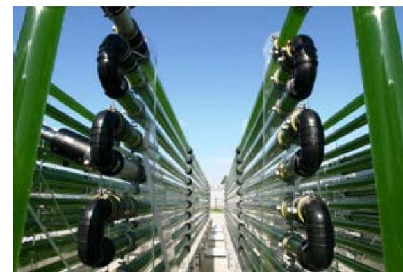
Figure 3. The energy cost to pump the algae through the bioreactor is very significant for the tubular system [3]
