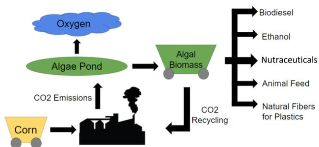
Figure 1. Flowchart of the proposed co-location of algae farm and ethanol plant
