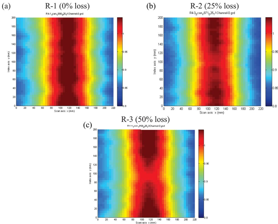
**FIGURE 5.** C-scan MFL images in the same color scale for rebar samples (a) R-1, (b) R-2 and (c) R-3, respectively.
