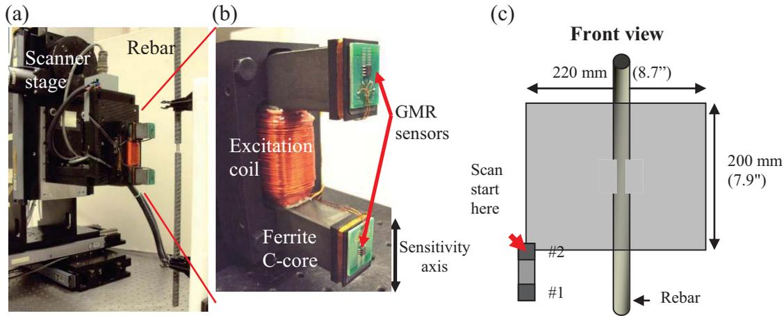
**FIGURE 3.** Experimental setup for performing MFL scans on the rebar samples. (b) Close-up of the MFL sensor probe. It consists of an electromagnet to apply magnetizing field, and two GMR sensors to detect the vertical component of leakage field at the pole-piece of the electromagnet. (c) A schematic diagram showing the size and coverage of the raster scans over the rebar samples. The perpendicular distance between the probe and rebar is 2.5" (63.5 mm).
