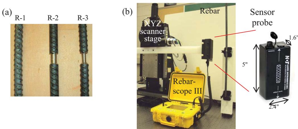
**FIGURE 2.** (a) Standalone rebar samples. Samples R-2 and R-3 were machined to produce artificial defects of 25% and 50% material loss, respectively. (b) Experimental setup for EC scans on the rebar samples using a commercial EC-based instrument. The outer dimensions of the sensor probe are shown in the inset.
