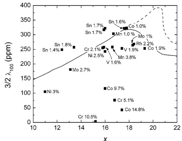
FIG. 2. Saturation magnetostriction ( $3/2 \lambda_{100}$ ) of ternary alloys (Fe<sub>100-x-y</sub>Ga<sub>x</sub>X<sub>y</sub> with X=V, Cr, Mn, Co, or Rh including previously reported Ni, Sn, and Mo) vs Ga content  $x$  (see Ref. 5). The lines are guides to the eye for the binary alloy (see Fig. 4): solid, quenched; dashed, quenched.
