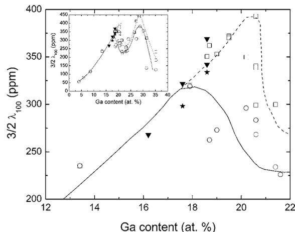
FIG. 4. Saturation magnetostriction vs Ga content for the  $\text{Fe}_{100-x}\text{Ga}_x$  system, with and without C additions. The inset shows the saturation magnetostriction between 4 and 35 at. % Ga. The lines are guides to the eyes: solid, unquenched; dashed, quenched.  $\circ$  Fe-Ga, unquenched;  $\square$  Fe-Ga, quenched;  $\blacktriangledown$  Fe-Ga-C, unquenched; and  $\star$  Fe-Ga-C, quenched.
