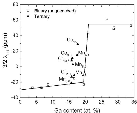
FIG. 3. Saturation magnetostriction ( $3/2 \lambda_{111}$ ) for the Fe-Ga binary system ( $\square$ ) and ternary additions (Cr, Mn, or Co) to the binary ( $\blacktriangle$ ). The line is a guide to the eyes.
