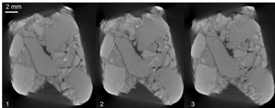
**Figure 6. X-ray high resolution tomography cross-sectional images of stripped HMA sample.**
