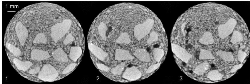
Figure 9. X-ray high resolution tomography cross-sectional images for FAC sample (aggregates of three different sizes [4.75-mm, 300- $\mu\text{m}$ , and 600- $\mu\text{m}$ ] floating in asphalt).
