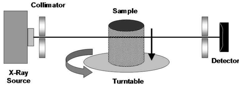
**Figure 2. Schematic of X-ray computed tomography system.**
