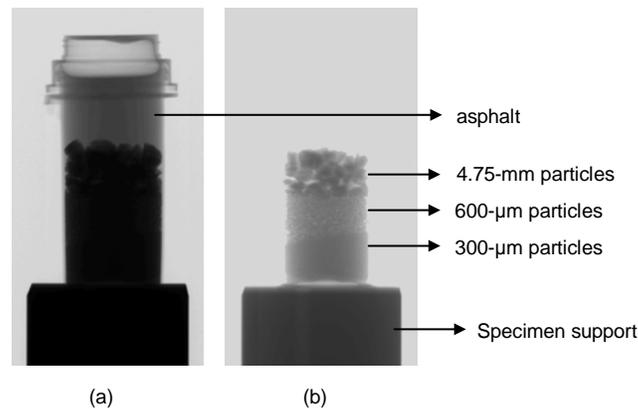
**Figure 7. X-ray shadow images of FAS sample: (a) 80-kVp, 0.10-mA; (b) 120-kVp, 0.40-mA.**
