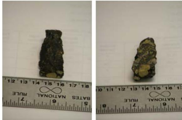
**Figure 5. Front and back views of stripped HMA sample used in this study.**
