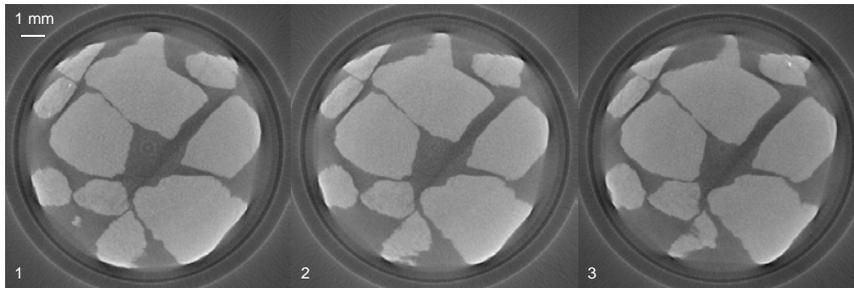
Figure 10. X-ray high resolution tomography cross-sectional images for CA sample (aggregates of three different sizes [12.7-mm, 9.5-mm, and 4.75-mm] floating in asphalt).
