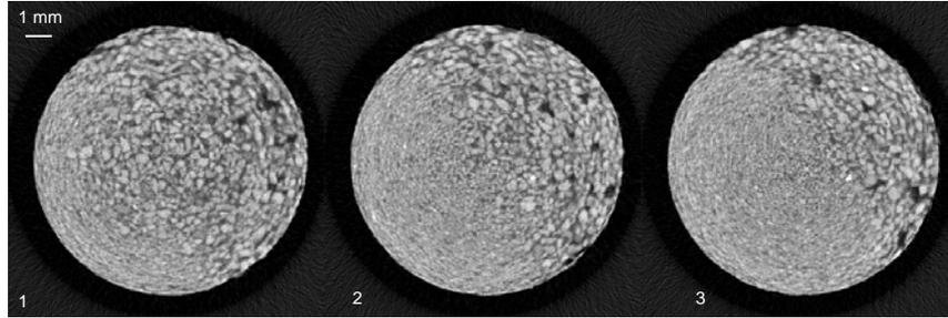
Figure 8. X-ray high resolution tomography cross-sectional images for FAS sample at the interface between 300- $\mu\text{m}$  particles and 600- $\mu\text{m}$  particles.
