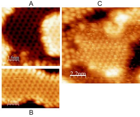
FIG. 6. (Color online) STM images showing the  $\sqrt{3}$  structure in islands and holes, after preparation using different conditions. (a) and (b) Prepared by deposition at 500 K, followed by 10 min anneal.  $V_T = -1.0$  V and  $I_T = 2$  nA. (c) Prepared by deposition at 600 K, followed by 2 min anneal.  $V_T = -1.0$  V and  $I_T = 0.2$  nA.
