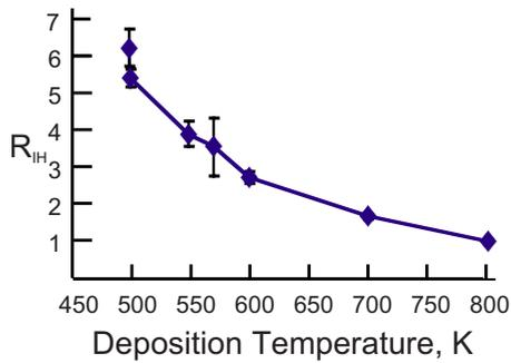
FIG. 3. (Color online)  $R_{IH}$  as a function of deposition temperature. The sample was held for 1 min at  $T_{dep}$  after deposition finished, with the exception of the first point. There,  $R_{IH}=6.2$  at 500 K, and the ratio was measured immediately after deposition. Values are averages over multiple images, and error bars are standard deviations. If no error bars are visible, they are obscured by the symbol.
