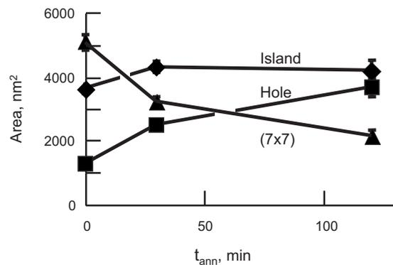
FIG. 5. Graph illustrating the change in areas of Si(111)- $7 \times 7$  phase (triangles),  $\sqrt{3}$  islands (diamonds) and  $\sqrt{3}$  holes (circles) with annealing time at 600 K. Values are averages over multiple images and error bars are standard deviations. Most error bars are obscured by the symbols.
