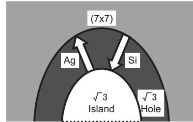
FIG. 9. Schematic illustration of the growth of a hole around a  $\sqrt{3}$  island.
