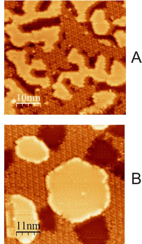
FIG. 7. (Color online) STM images of islands, showing rims.  $V_T = -1.0$  V and  $I_T = 0.2$  nA. (a) Prepared by deposition at 615 K, annealed 2 min.  $50 \times 50$  nm<sup>2</sup>. (b) Prepared by deposition at 800 K, annealed 2 min.  $65 \times 65$  nm<sup>2</sup>.
