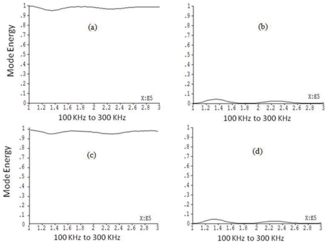
**FIGURE 5.** Energy transmission coefficients for configuration in Fig.(1b): a) A0 to A0, b) A0 to S0, c) S0 to S0, and d) S0 to A0. No appreciable reflection is observed.
