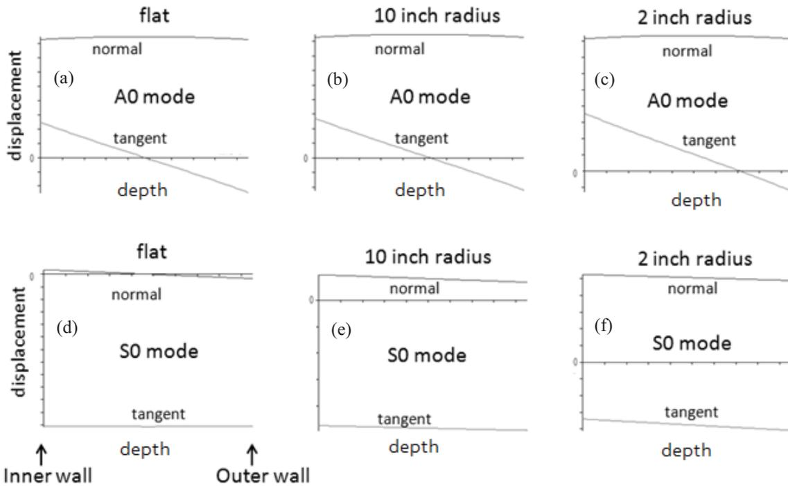
**FIGURE 3.** Comparison of tangential and normal 100 KHz motion profiles as function of depth through 3/16" shell wall for: a) A0 flat plate, b) A0 10 inch radius, c) A0 2 inch radius, d) S0 flat plate, e) S0 10 inch radius, f) S0 2 inch radius.
