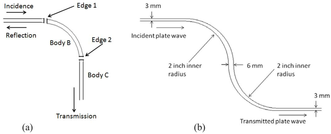
FIGURE 1. Problem configurations: transmission at a) circular curved section, b) tapered section.
