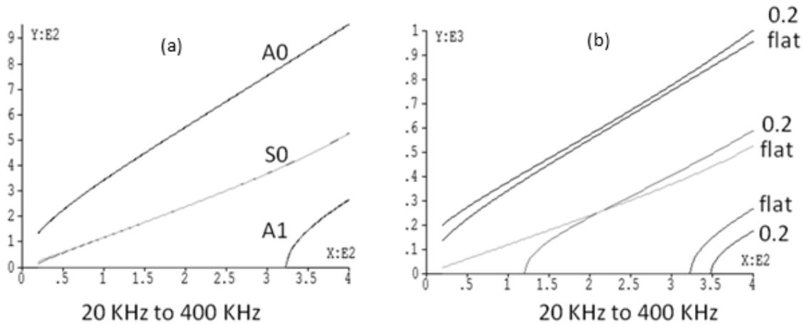
**FIGURE 2.** Dispersion relation for guided modes in 3/16 inch thick cylindrical shell: overlay of a) flat plate and 2 inch inner wall radius, b) flat plate and 0.2 inch inner wall radius. Vertical axis is circumferential wave number at the inner radius.
