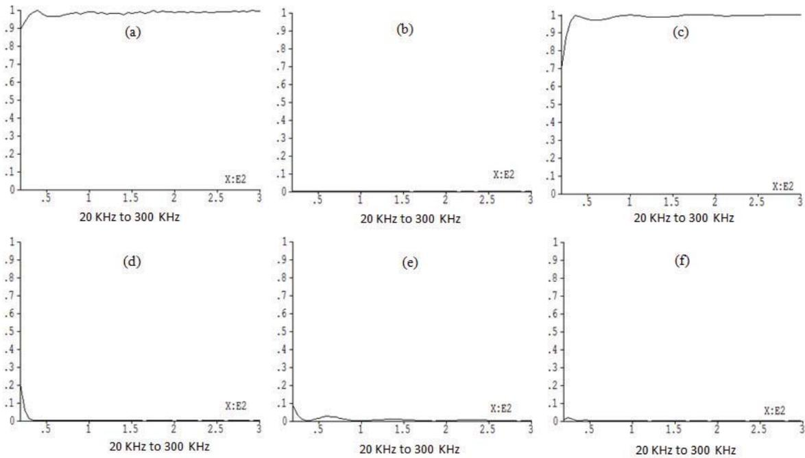
**FIGURE 4.** Energy transmission and reflection coefficients for: a) A0 to A0 transmission, b) A0 to A0 reflection, c) S0 to S0 transmission, d) S0 to S0 reflection, e) A0 to S0 or S0 to A0 transmission, f) A0 to S0 or S0 to A0 reflection.
