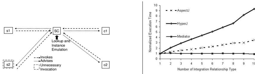
Fig. 15. Runtime Object Structure for an Aspect-based implementation (left) and Performance Curve for AspectJ, HyperJ, and Mediator-Based Design (right)
