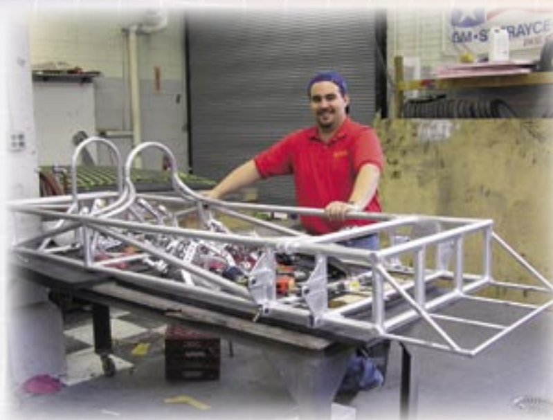
Justin Steinlage, director of Iowa State's Team PrISUm, shows the frame for Iowa State's entry in the 2005 North American Solar Challenge. Named Fusion, the new car is designed to be more aerodynamic and lighter weight than past entries.
