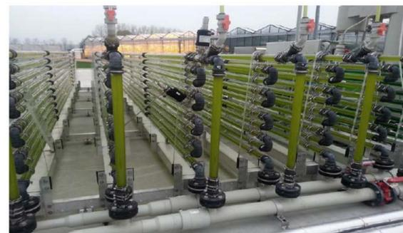
Figure 2. Example of a photobioreactor<sup>[3]</sup>.
