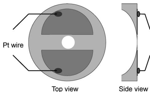
FIG. 1. Schematic diagram of specimens for the electric field *in situ* TEM study.
