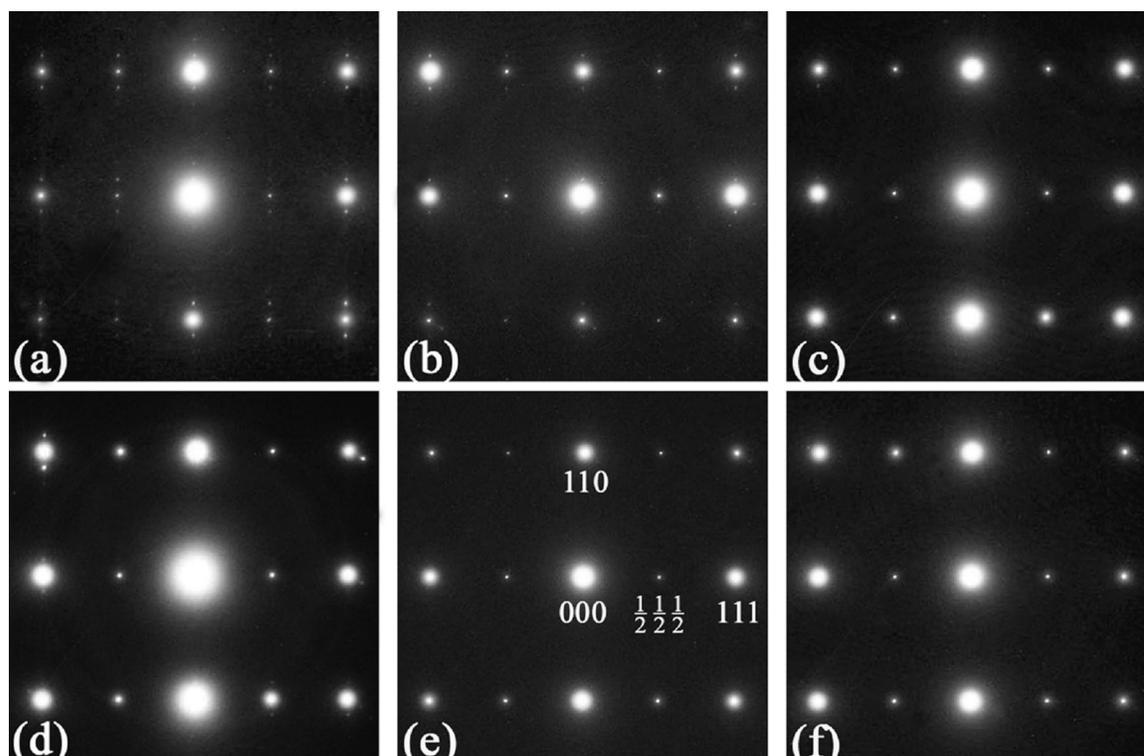
FIG. 4. Evolution of the  $\langle 112 \rangle$  selected area diffraction pattern under applied electric fields in PZST 45/6/2. (a) Original state, (b) 48, (c) 56, (d) 40, and (e) 56 kV/cm, and (f) field removed.
