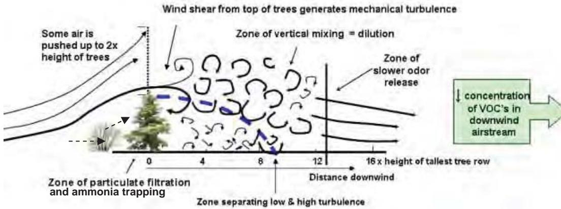
Figure 1. Generalized schematic of VEB odor mitigation dynamics. Note that the magnitude of dynamics listed in text above and shown here are site and VEB specific.
