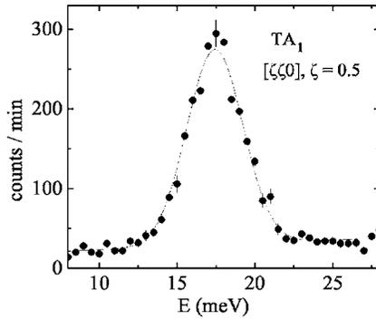
FIG. 1. Observed neutron group for the  $[\xi\xi0]$   $TA_1$  branch at the zone boundary ( $N$ -point) for  $Fe_{90}Be_{10}$ .  $\xi$  is the reduced wave vector in units of  $2\pi/a$ .
