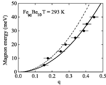
FIG. 4. Room temperature spin wave dispersion relation along [001] for  $\text{Fe}_{90}\text{Be}_{10}$ . The solid curve shows the relation  $E=Dq^2$  for  $D=210 \text{ meV \AA}^2$ , while the dashed curve shows the dispersion relation observed at small values of  $q$  for pure Fe with  $D=280 \text{ meV \AA}^2$ . Units of  $q$  are in  $\text{\AA}^{-1}$ .
