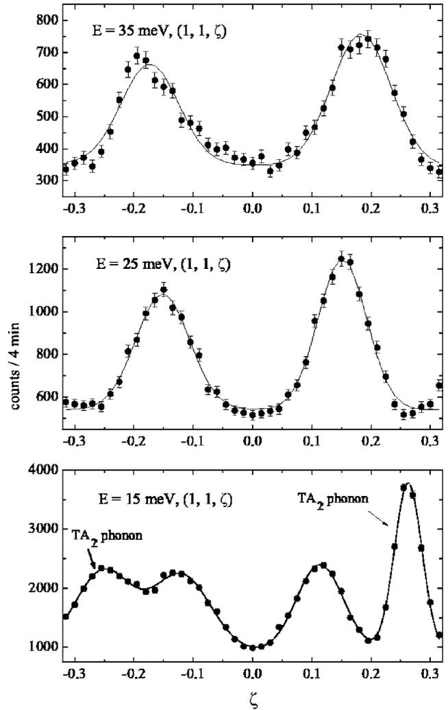
FIG. 3. Room temperature constant- $E$  scans at 15, 25, and 35 meV for  $Fe_{90}Be_{10}$  along the  $[001]$  direction.
