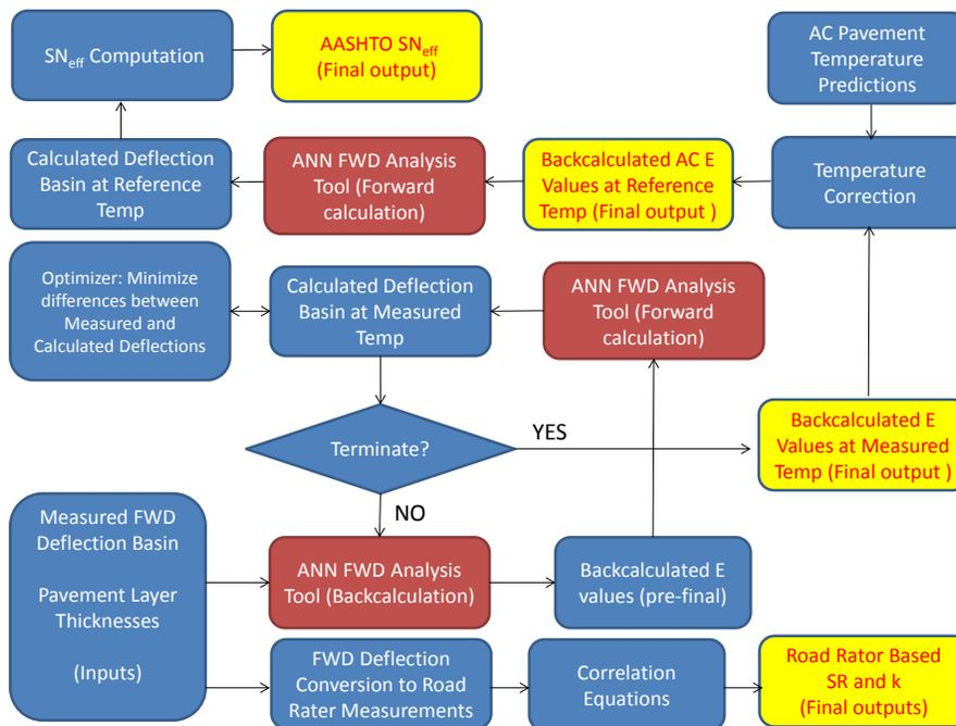
**FIG. 2. I-BACK analysis flow chart: flexible pavement module**
