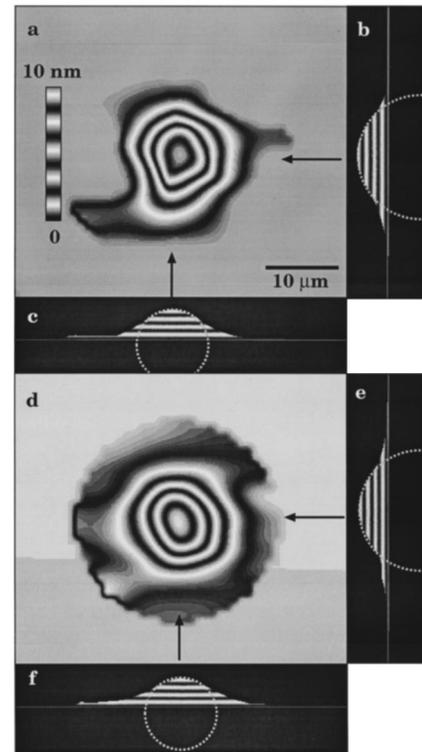
FIG. 3. Top view and side view images from particles (b) and (e) [see Fig. 1(a)]. The superimposed circle is 8.5 nm in radius of curvature in (b) and (e) and 5.0 nm radius of curvature in (c) and (f). The scale bar in (a) is 10 nm.
