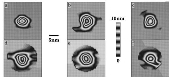
FIG. 2. Panel of six different reconstructions of the same tip from four different gold particles [numbered in Fig. 1(a)]. The contour map shows approximately 2 nm of vertical height change between each pair of black and white bars.
