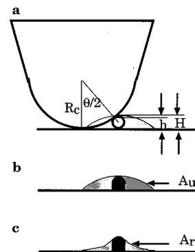
FIG. 4. (a) Model of the key components for the cross sectional image reconstruction components. (b) The approximate unreconstructed cross section  $A_u$  due to the tip's apex mapping out an image of the smaller G-wire DNA (black silhouette). (c) The reconstructed cross section  $A_r$  when the shape of the tip is removed from (b). The black silhouette in the middle of (b) and (c) is the cross sectional shadow of the G-wire DNA expected for an ideal (delta function) tip.
