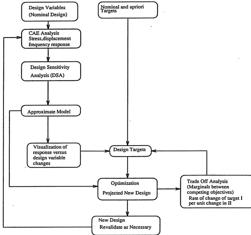
Figure 1: FLOW CHART FOR STRUCTURAL/ACOUSTIC ANALYSIS
