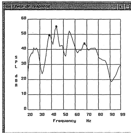
Figure 2: SPL AT THE DRIVERS EAR, FRONT WHEELS IN PHASE (*fwip*) CASE
