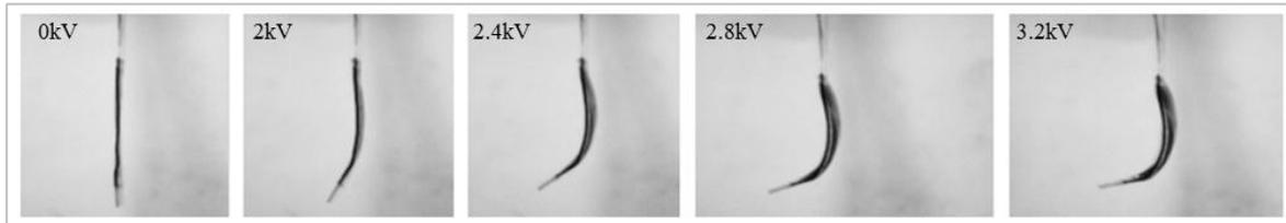
Figure 3. Deformed shape of a 4-stack configuration actuator under applied voltage range of 0-3.2kV
