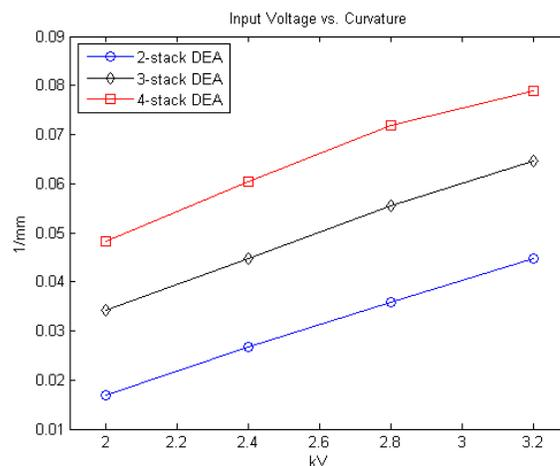
Figure 4. The experimentally evaluated bending curvatures for different stack configurations of actuators with single stiffener under a range of applied voltage potential.
