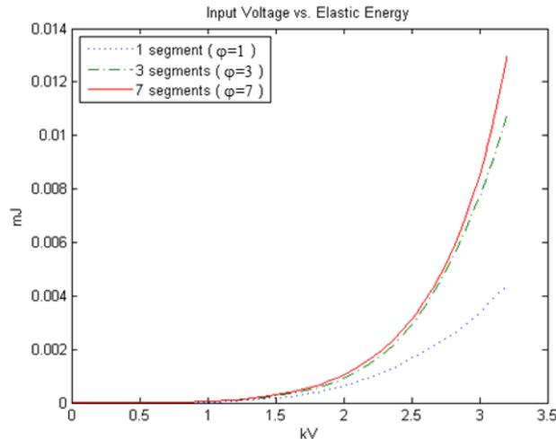
Figure 7. The FEM results of the variation of the elastic strain energy with splitting stiffeners into narrower segments.
