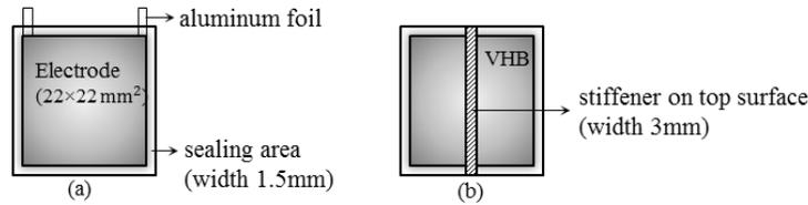
Figure 1. Sketches of DEA samples. (a) Top view of unit-cell DEA structure and its measurement with (b) single strip configuration stiffener in the middle on the surface.
