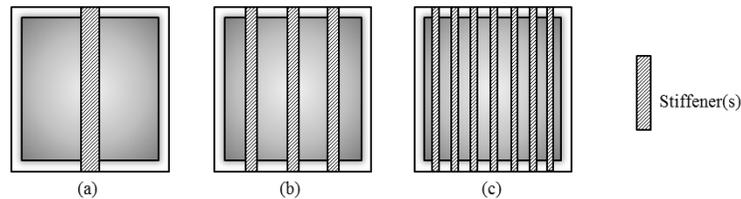
Figure 5. Sketches of stiffeners periodicity variation by splitting the stiffener(s) into distributed segments while maintaining the total stiffener width to keep the entire stiffness. (a) 1 segment ( $\phi=1$ ), (b) 3 segment ( $\phi=3$ ), (c) 7 segment ( $\phi=7$ ).
