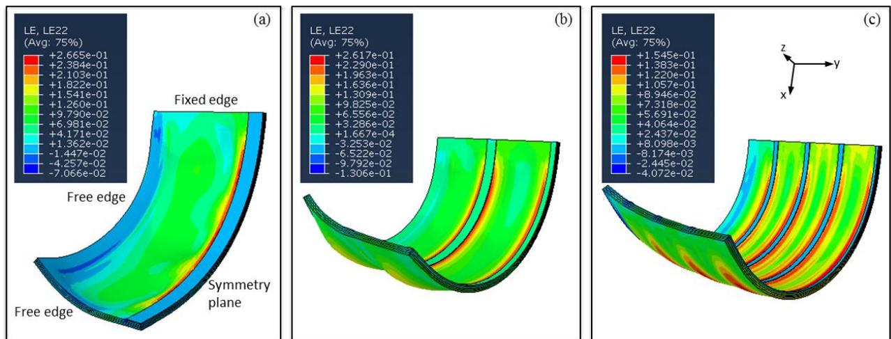
Figure 6. FEM results of the in-plane strain along the stiffeners direction, shown on the deformed mesh for different  $\phi$ ; (a)  $\phi=1$ , (b)  $\phi=3$ , (c)  $\phi=7$ . The total actuated volume within the span of the actuator increases with the refinement of the stiffener,  $\phi$ .
