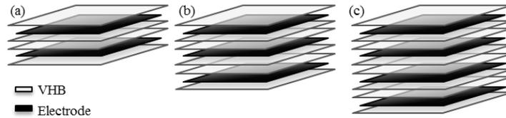
Figure 2. Sketches of DEA samples fabrication with side view of different stack configurations. (a) 2-stack (b) 3-stack (c) 4-stack.
