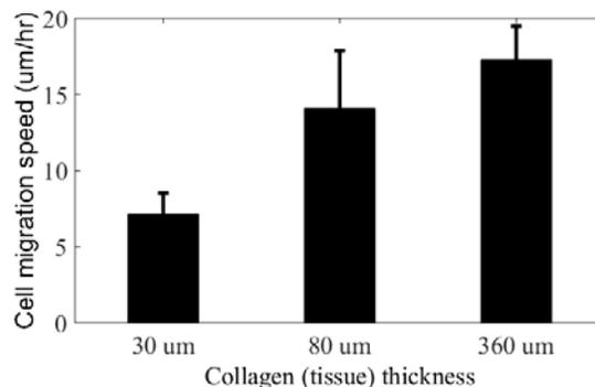
Fig. 6. Thickness (volume) effect on the migration speed: the 2<sup>nd</sup> generation devices with chamber heights of 30 m and 80 μm. A large gel with a height of 360 μm. The cell migration speed in 30 μm thick microtissue is half of that in 80 μm thick microtissue, which is close to the migration speed in the 360 μm thick tissue.
