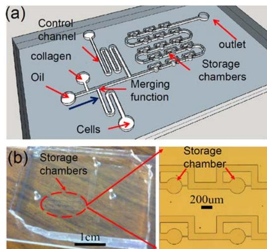
Fig. 1. (a) Sketch of the droplet microfluidic device for generating 3D microtissues: Each storage chamber (a cylinder with a radius of  $180 \mu\text{m}$  and height of  $30$  or  $80 \mu\text{m}$ ) has one 3D microtissue containing single or multiple cells; (b) photo of a fabricated chip with 15 storage chambers; (c) optical micrograph showing the storage chambers.
