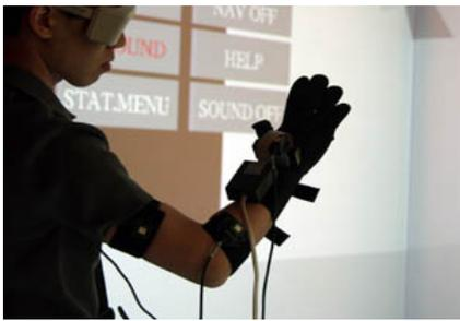
Figure 2: 5DT Data Glove 5-W and trackers
